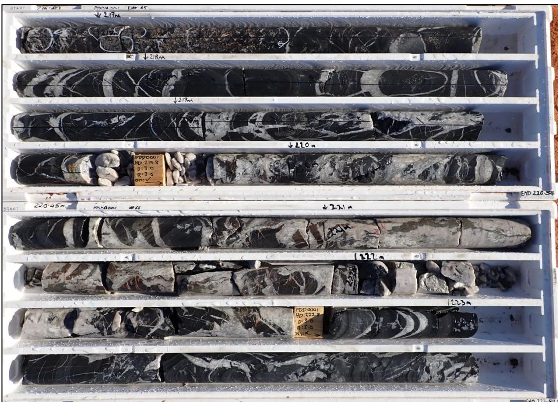
**Figure 2:** Core from PDD0001 showing quartz-carbonate veining and pyrite associated with the Grace/Bemm fault zone from 216.8m to 223.89m.
