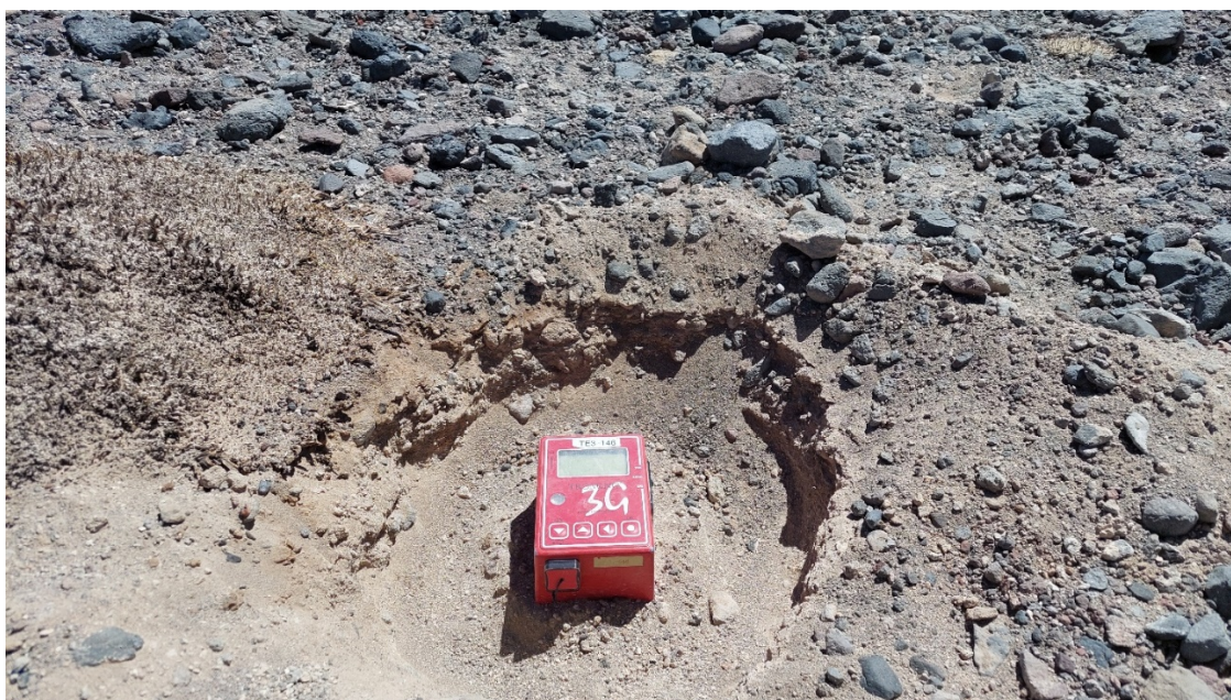
Figure 2 Tromino seismic equipment being used adjacent to the salt lake
