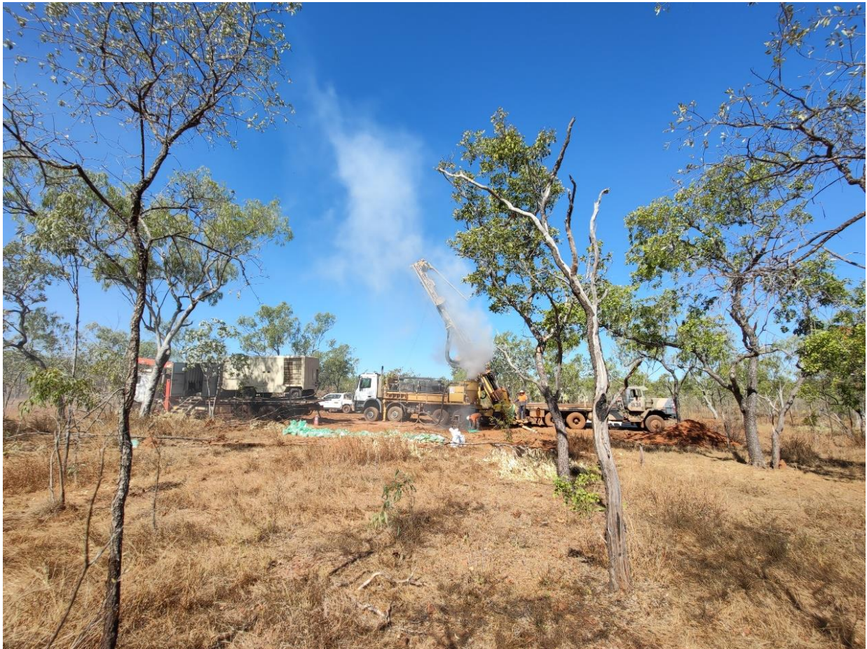
Figure 1: RC drill rig in operation at IP targets east of the Bluff Copper Deposit
