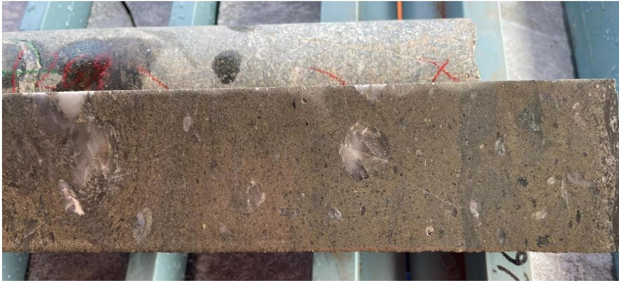
**Figure 7. Massive pyrite-pyrrothite breccia at 263.9 to 264.2m in drill hole NKLDD004 at the Fire Dragon 2 target.**
