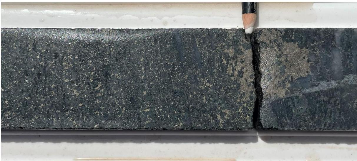
**Figure 8. Disseminated and remobilised sulphide in altered mafic (amphibolite) gneiss interpreted to represent deformed gabbro at 263.4 metres in NKLDD004.**
