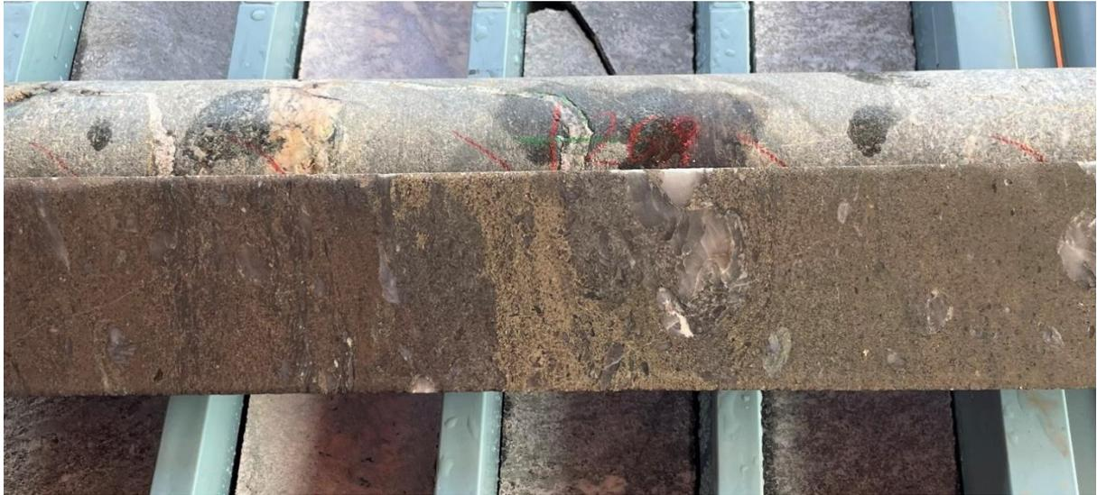
**Figure 5. 0.55m massive breccia sulphides intersected at 263.55m depth in drill hole NKLDD004 at the Fire Dragon 2 target.**
