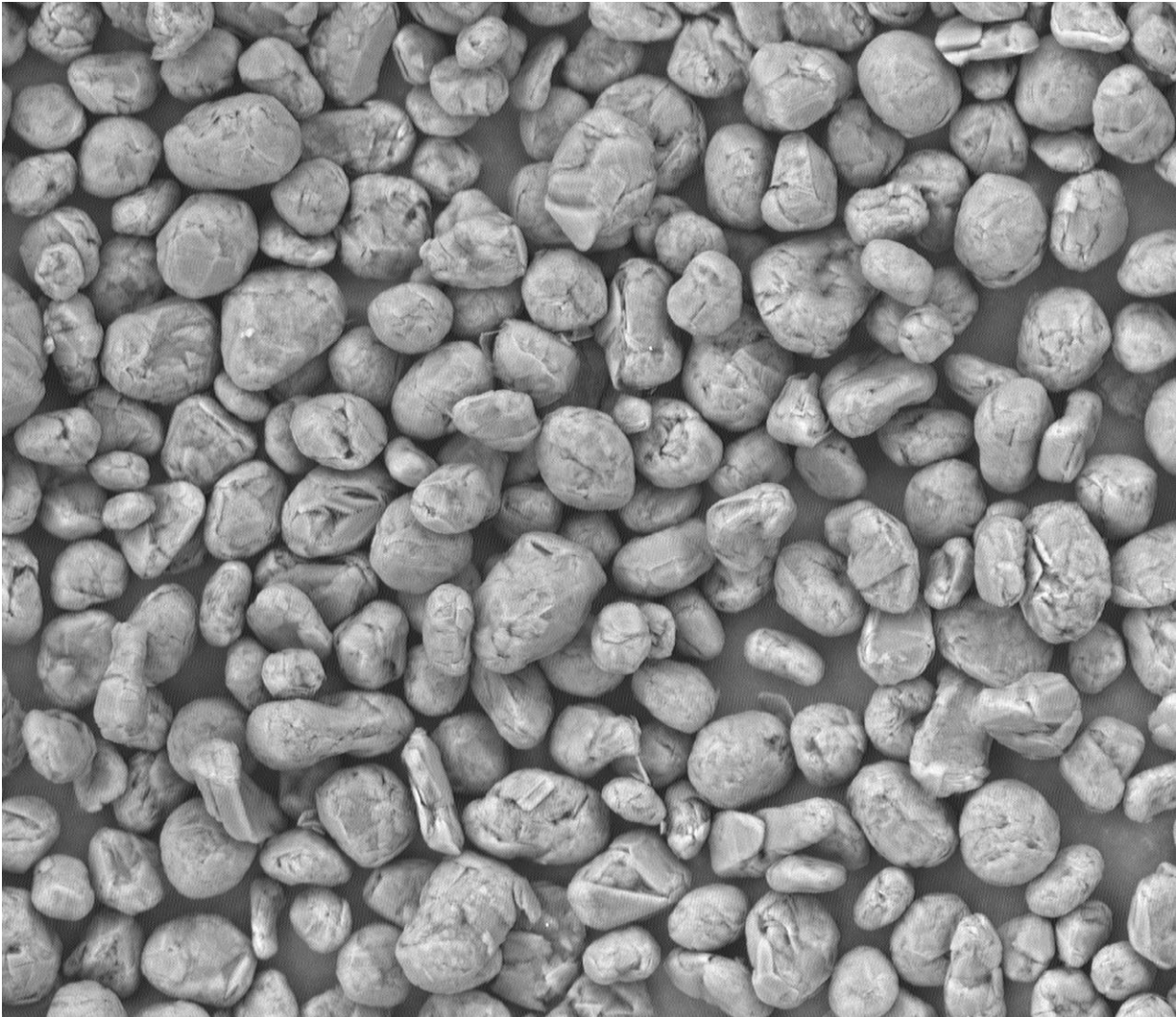
Picture 1: SEM image of 20 micron spherical graphite
