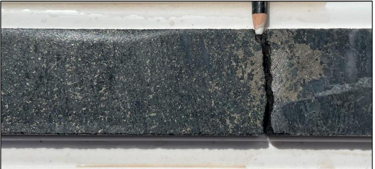
Figure 4. Disseminated and remobilised sulphide in altered mafic (amphibolite) gneiss interpreted to represent deformed gabbro at 263.4 metres in NKLDD004.
