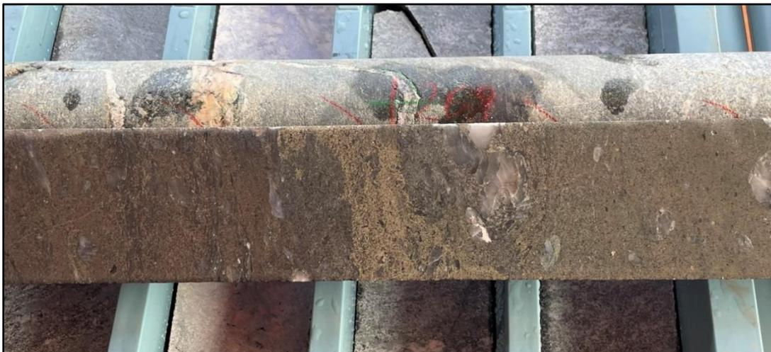
Figure 1. 0.55m massive breccia sulphides intersected at 263.55m depth in drill hole NKLDD004 at the Fire Dragon 2 target.
