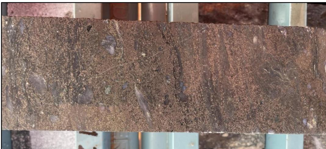
Figure 2. Massive pyrrhotite-chalcopyrite breccia at 263.65 to 263.9m in drill hole NKLDD004 at the Fire Dragon 2 target.
