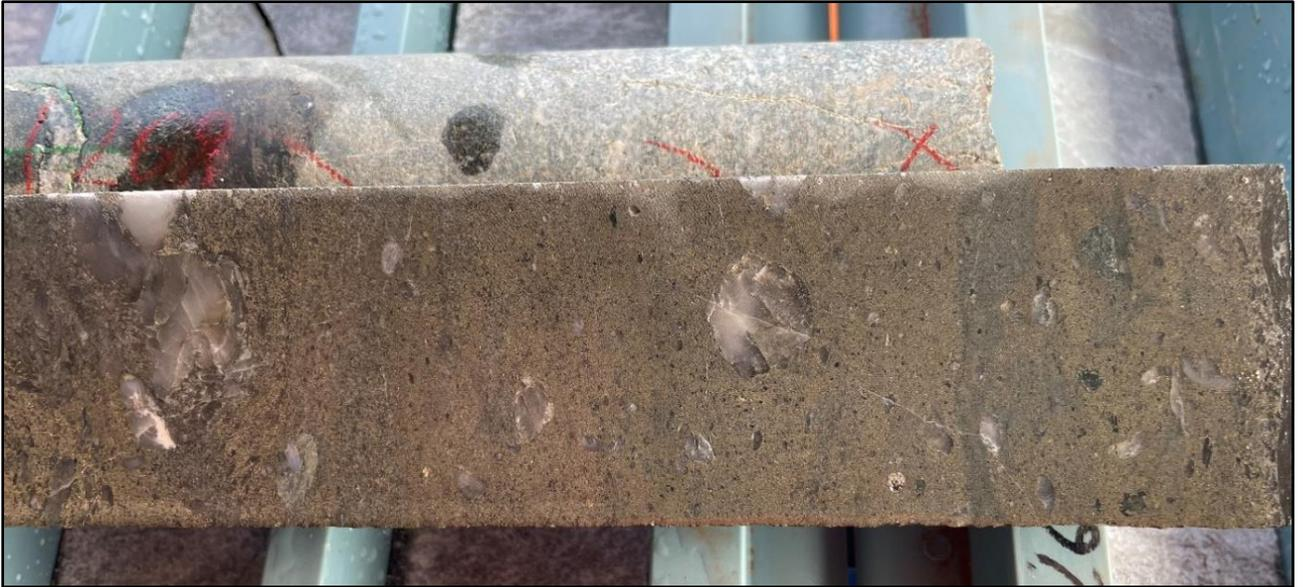
Figure 3. Massive pyrite-pyrrhotite breccia at 263.9 to 264.2m in drill hole NKLDD004 at the Fire Dragon 2 target.
