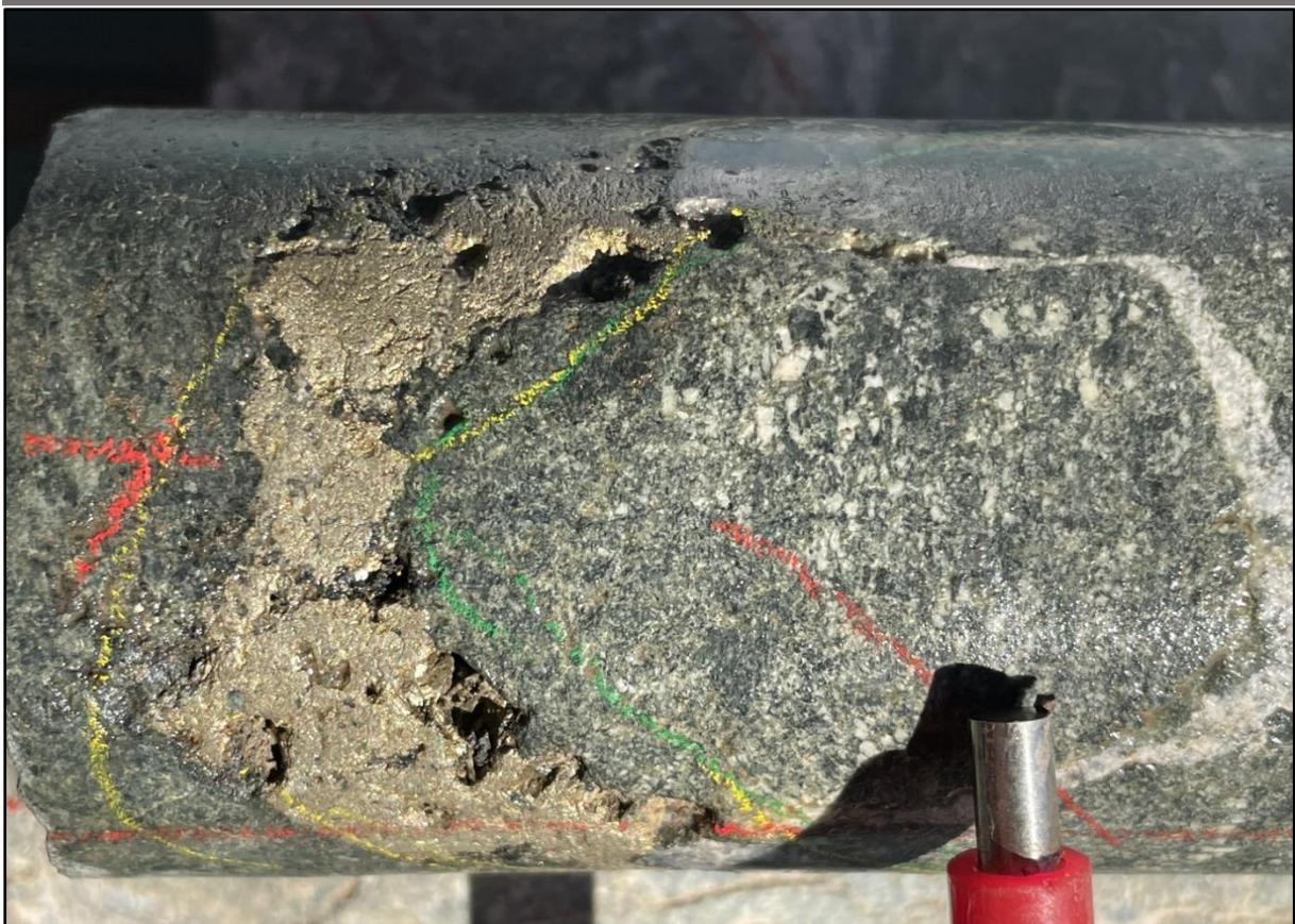
**Figure 5. Coarse remobilised sulphide in altered mafic (amphibolite) gneiss interpreted to represent deformed gabbro at 267.9 metres in NKLDD004.**
