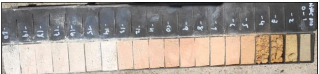
Figure 4: NVAC010 chip tray showing white sand at 13–17 m used for microscope photos
