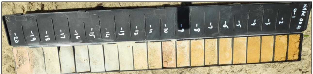
Figure 3: NVAC004 chip tray showing pale yellowish sand at 10–13 m used for microscope photos
