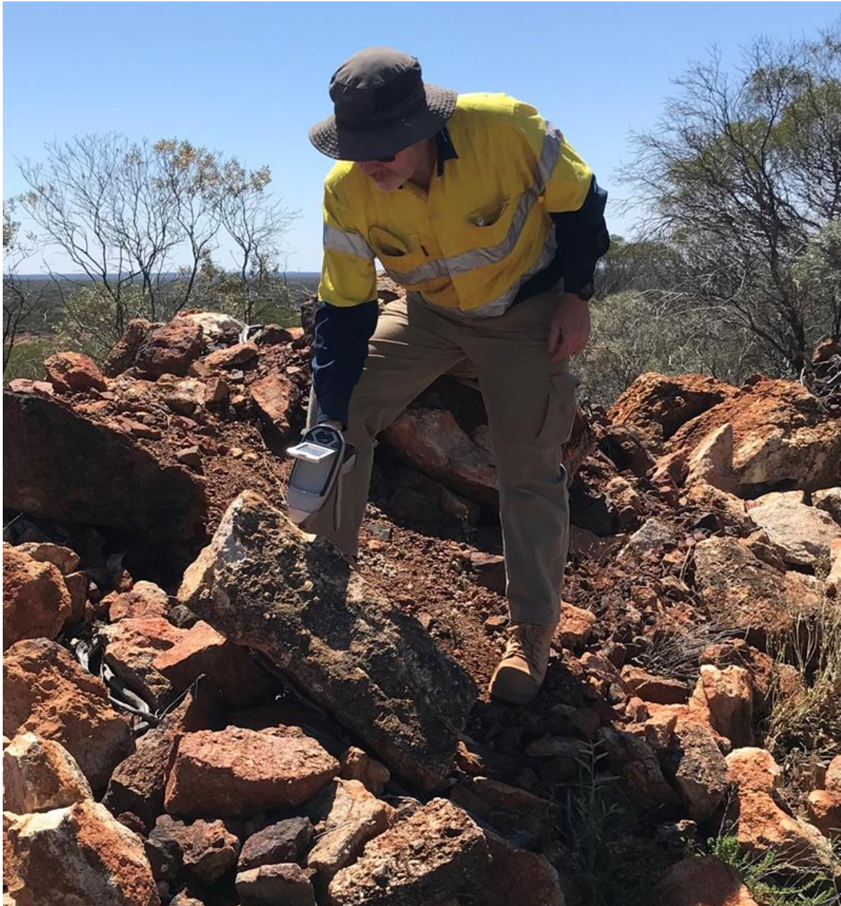
Photo 2: Pegmatite north of Mulgara, hand-held XRF analysis of lithium bearing minerals
