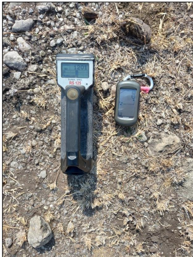
Figure 7: Ground Spectrometer surface reading of 1200 counts per second (CPS) Minjingu Project (822870mE/9589144mN)
