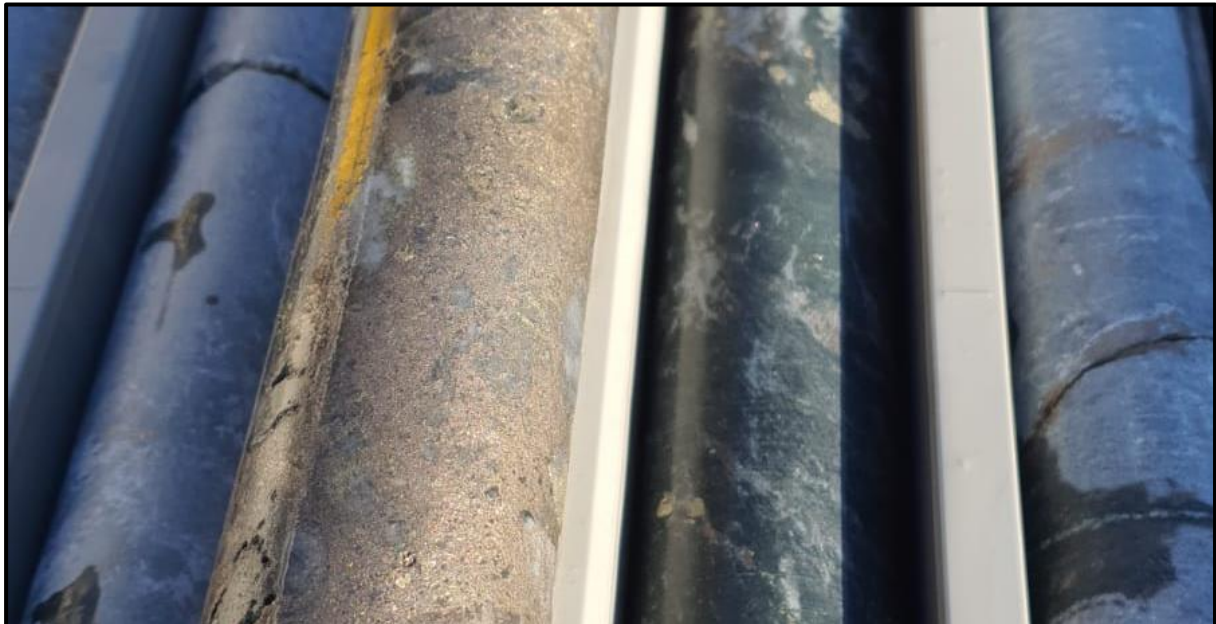
Figure 1 Semi massive and disseminated sulphide intersected by NDD0010 around 140m downhole. Hole size is NQ2.
