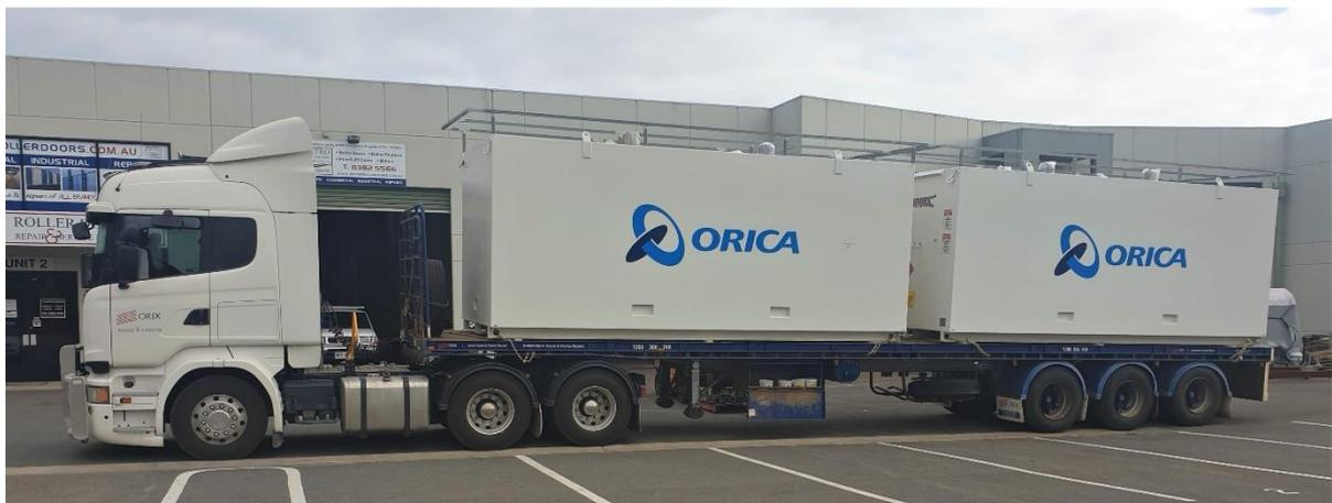
Fig 2. Two MagLok magazines (6M) being delivered to a client's site to be installed
