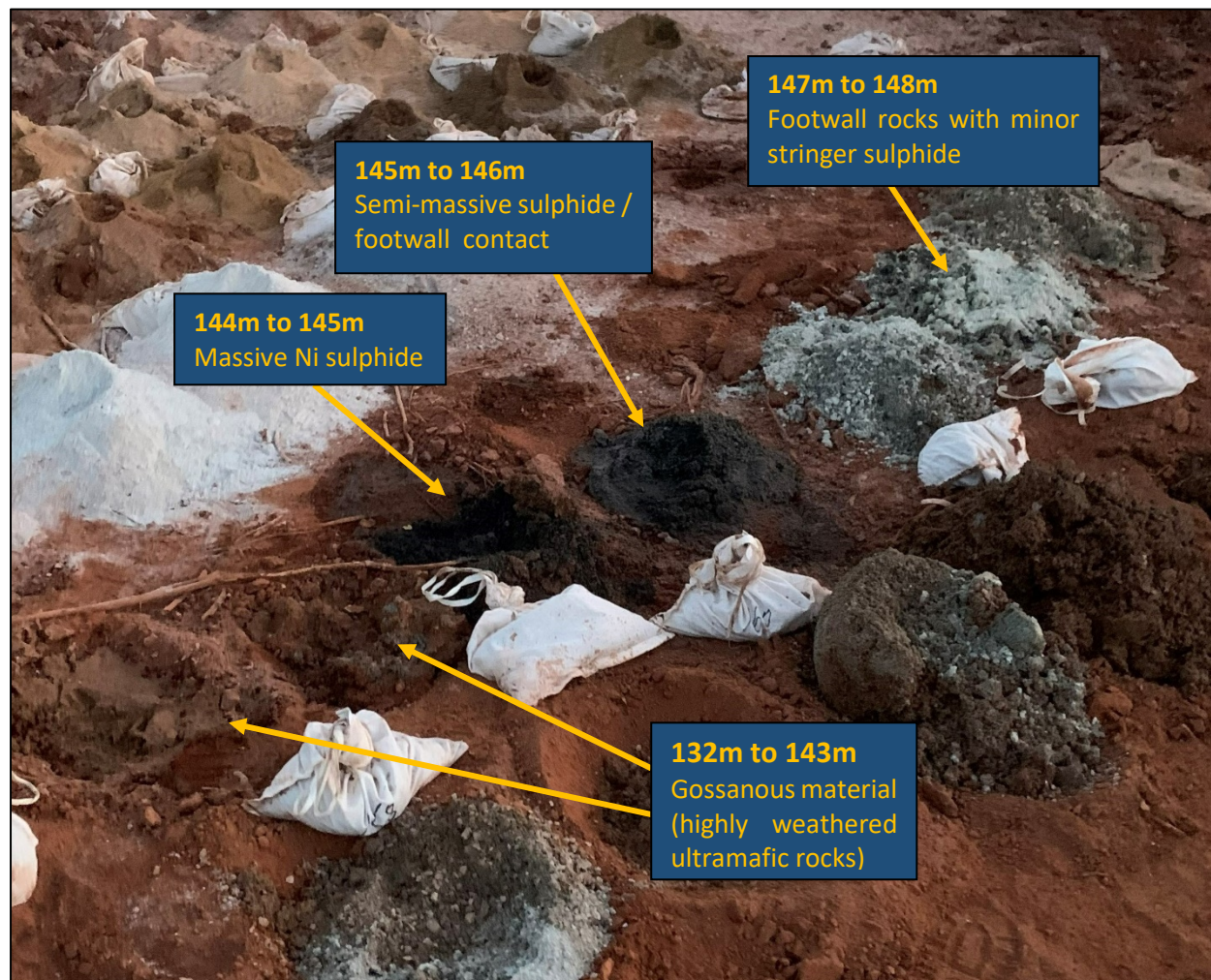
Figure 2. BVNC002 samples– nickel sulphide mineralisation highlighted
