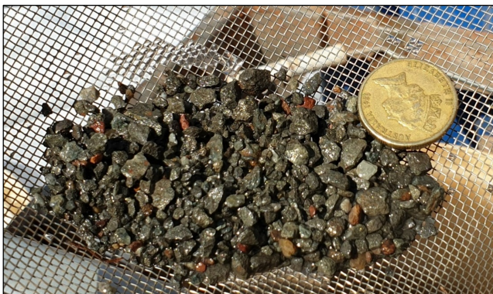
Figure 1. Massive nickel sulphides – BVNC002: 144m to 145m
