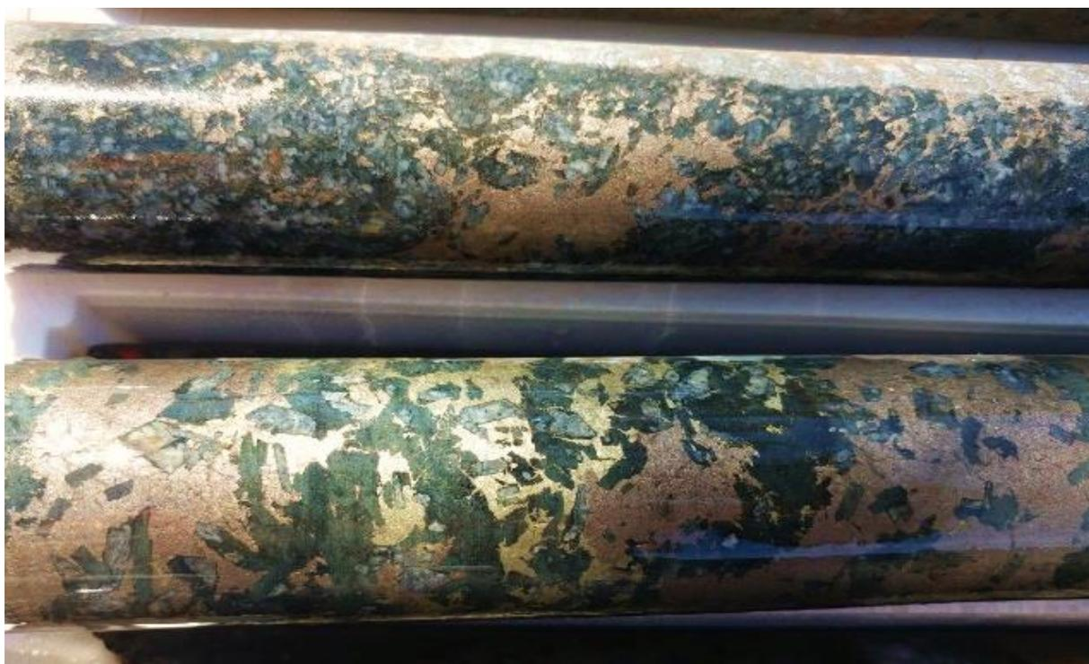
**FIGURE 3: 17MVRCD008 – SEMI-MASSIVE AND STRINGER PYRRHOTITE WITH CHALCOPYRITE (113M)**
