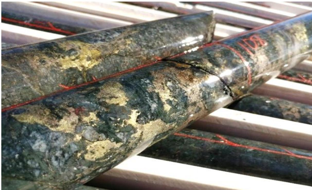
**FIGURE 2: 17MVDD003 – BASAL CONTACT WITH INTERSTITIAL CHALCOPYRITE AND PYRRHOTITE WITHIN VERY COARSE-GRAINED GABBRO (108M)**
