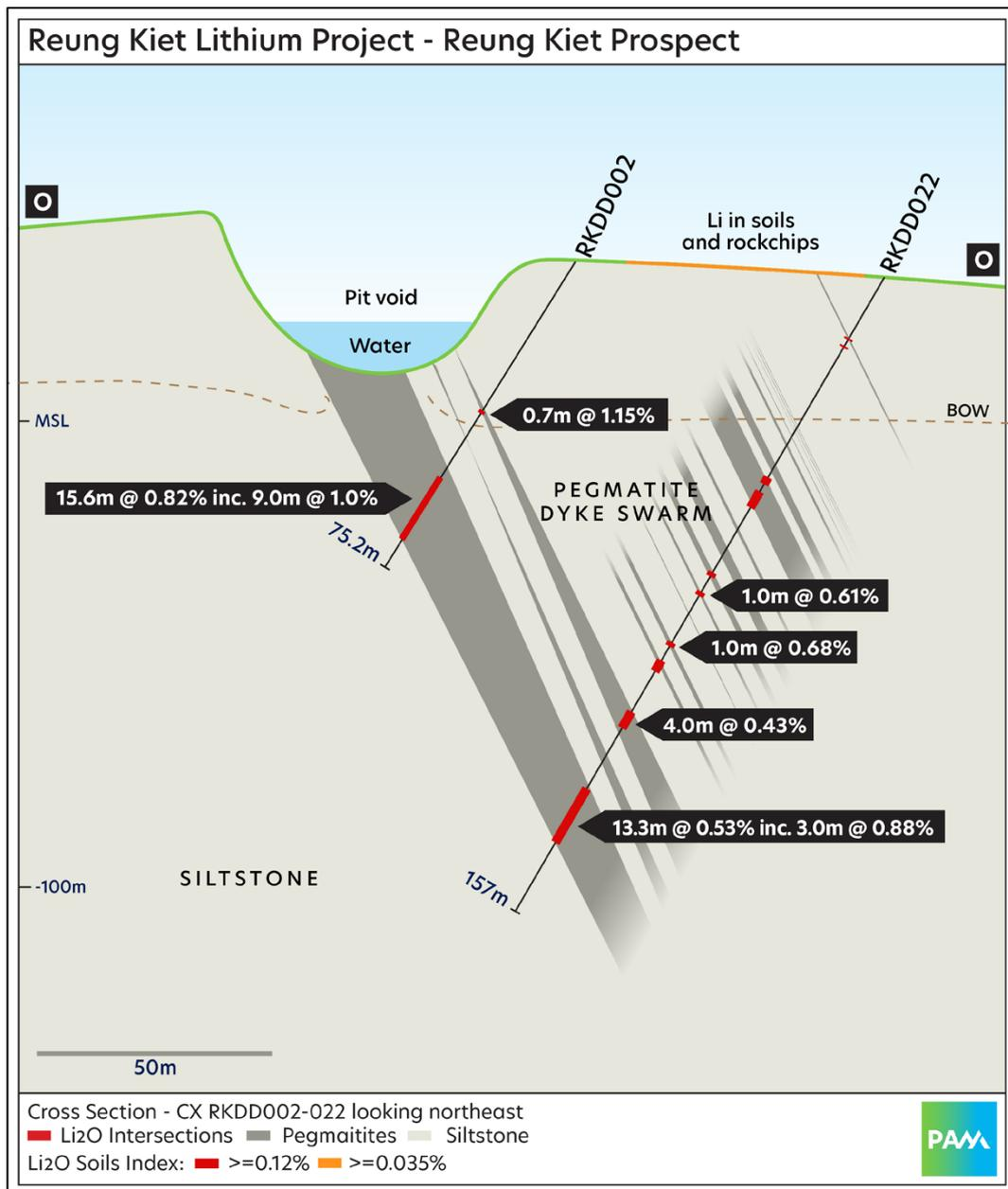
Figure 10. Section I showing RKDD002 and RKDD022
