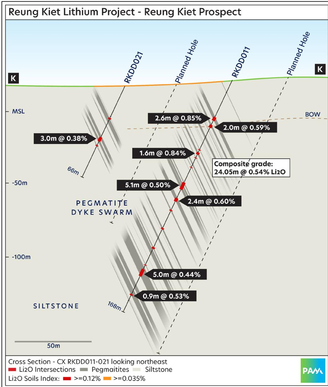
Figure 8. Section K showing RKDD011 and RKDD021
