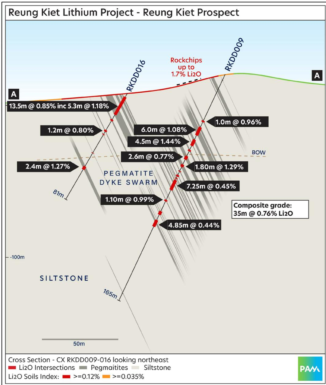
Figure 3. Section A showing RKDD009 and RKDD016.
