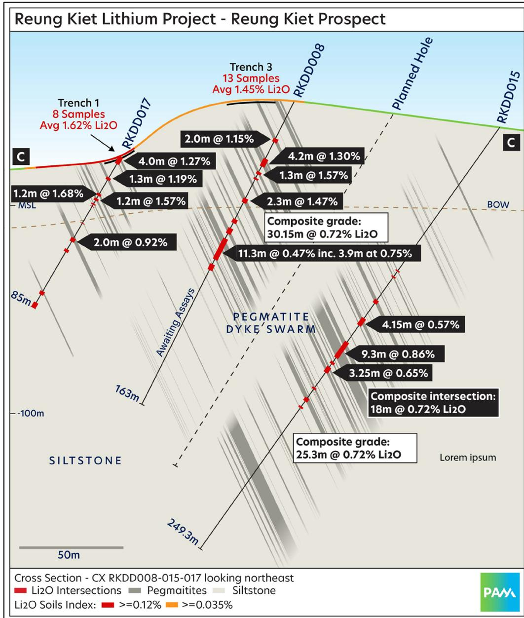
Figure 4. Section C showing RKDD008, RKDD017 and RKDD015
