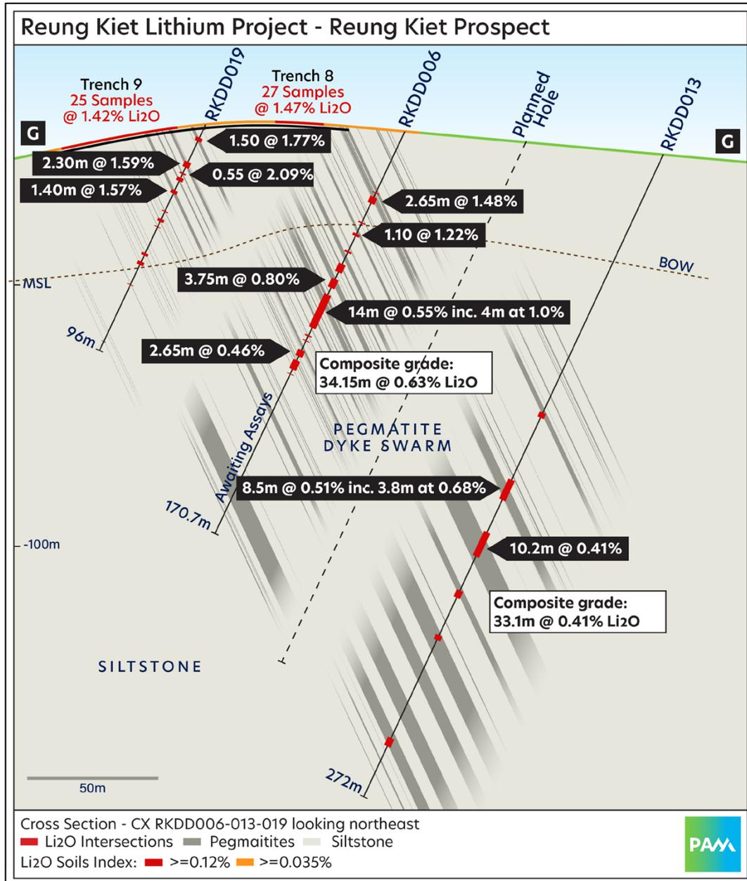
Figure 6. Section G showing RKDD006, RKDD013 and RKDD019
