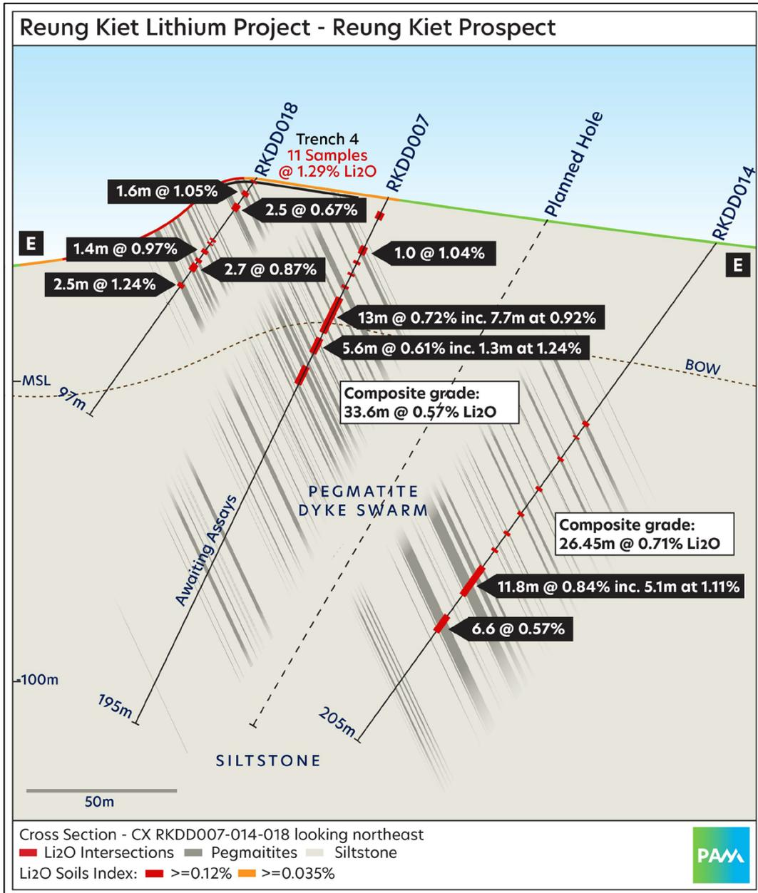
Figure 5. Section E showing, RKDD007, RKDD014 and RKDD018
