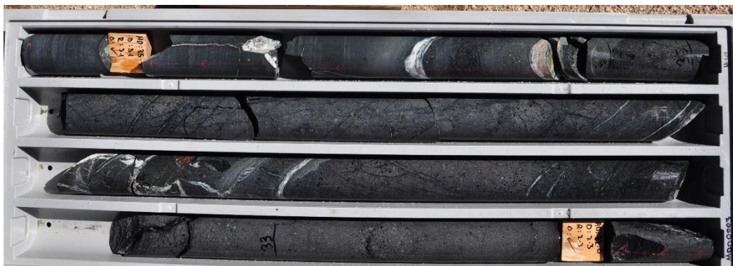
Figure 4: Drill core from MQD0003 between 32.7m to 35.1m. Sericitised and chloritised plagioclase-rich porphyritic diorite.
