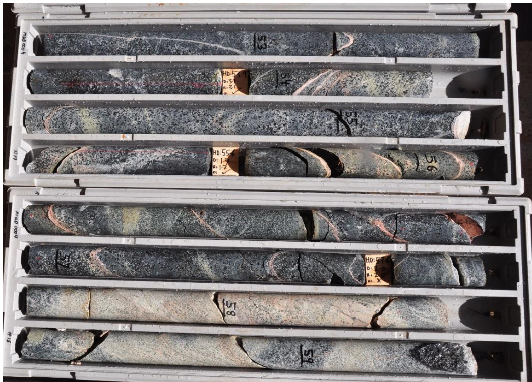
Figure 3: Drill core from MQD0004 displaying intense potassic alteration, from 52.5m to 59.5m
