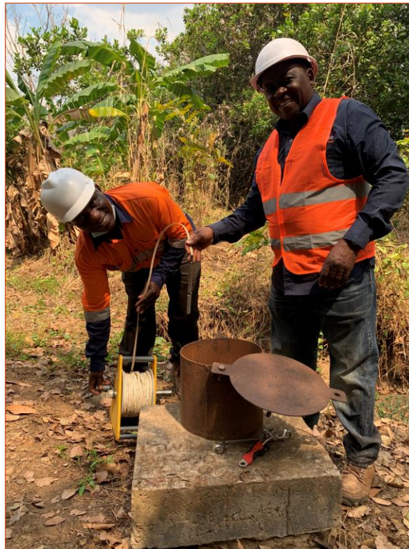
Figure 2: Water borehole monitoring on site.
