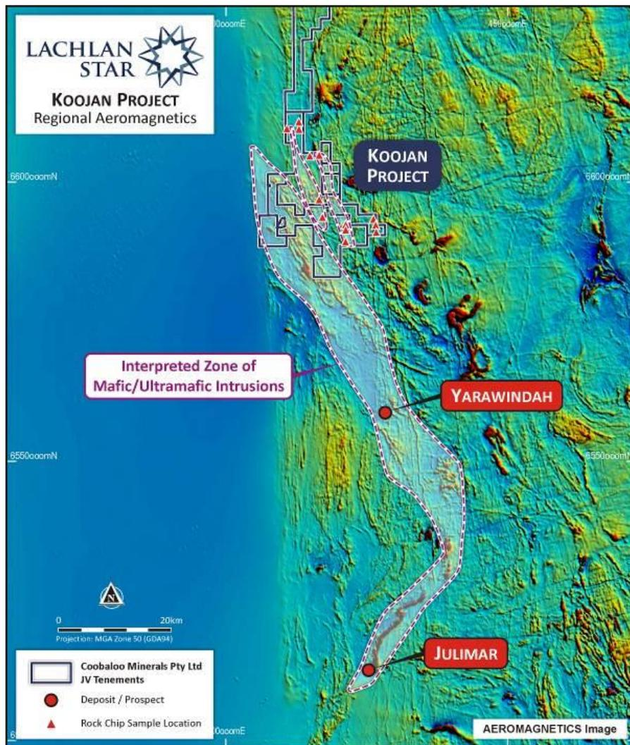
**Figure 2: Regional Airborne Magnetic Geophysical survey data**
