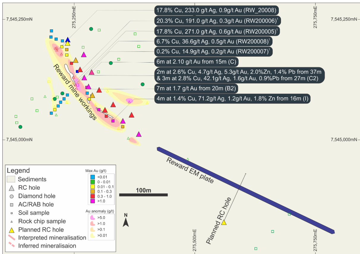
Figure 5: Map of Reward showing historic mine workings with best assay results and EM plate to the south with planned RC hole (ASX: 13 May 2010)
