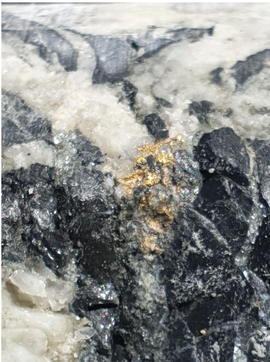
Plate 2: Visible Gold in diamond drill hole TND002 at 230.6 metres at Macnaughtan Prospect. Field of view approx. 50mm.
