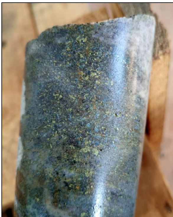
Figure 2 – Detail from CKDD003 exhibiting silicified metagranodiorite highly mineralised with chalcopyrite at 36m
