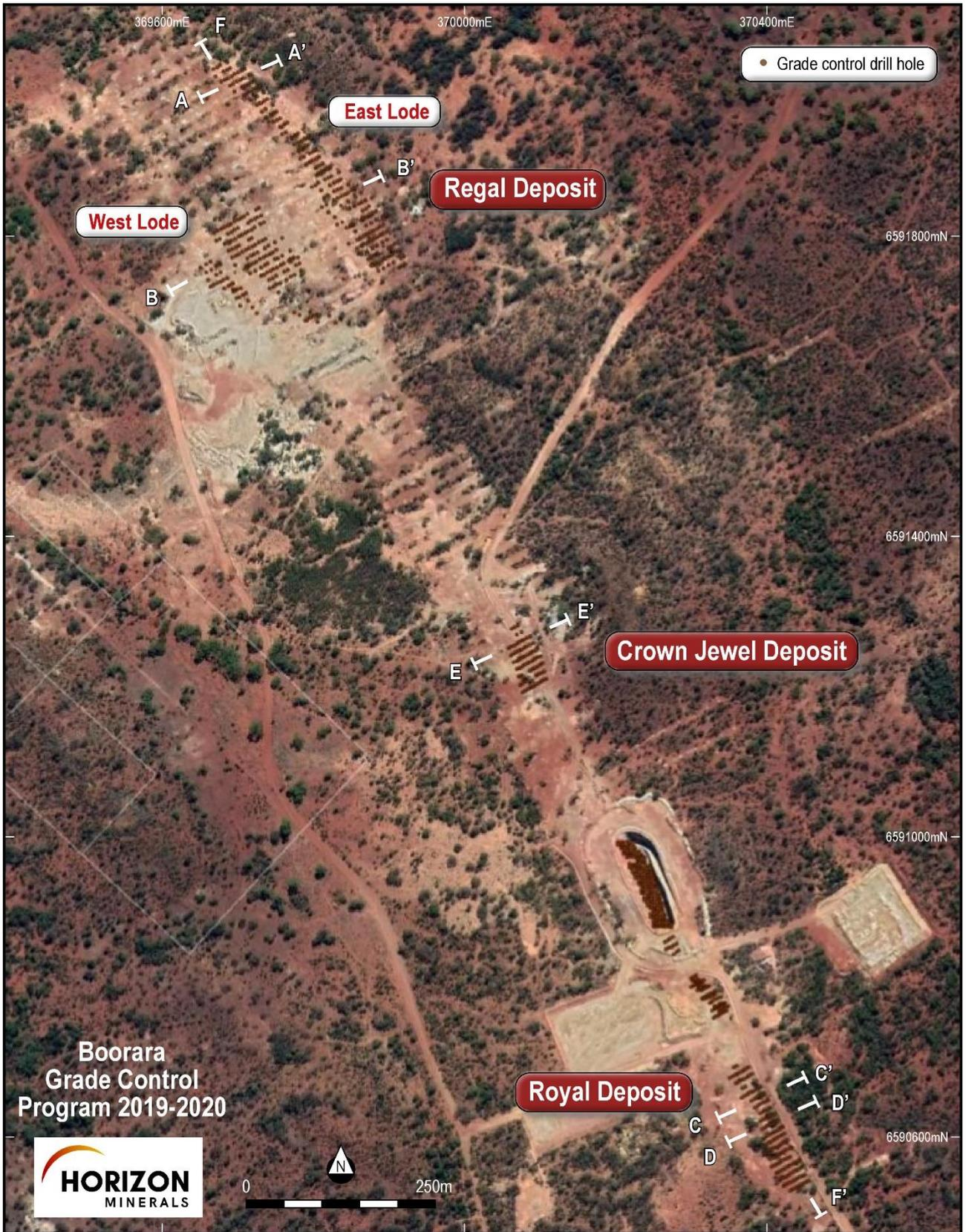
Figure 3: Boorara grade control drilling plan and cross section locations
