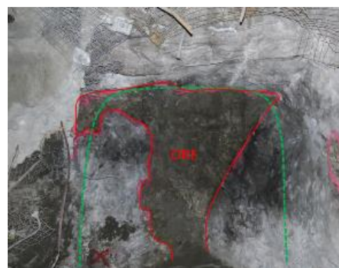
150 North ore drive with a face grade 2.8% Ni
