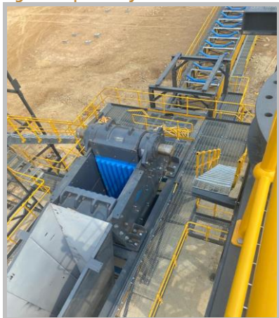
Figure 16 | Primary Crusher Installed
