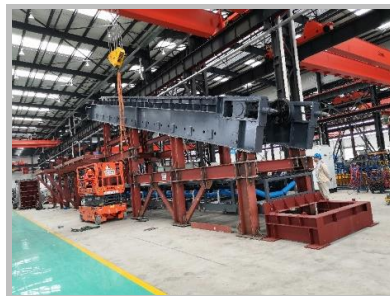
Figure 15 | Apron Feeder
