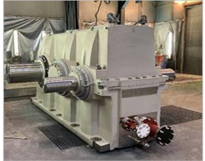
Figure 7 | SAG Mill Gear Box
