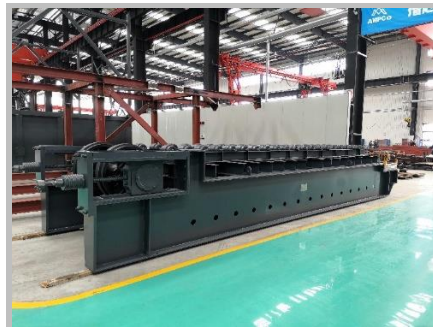
Figure 15 | Apron Feeder
