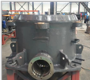
Figure 14 | Pebble Crusher
