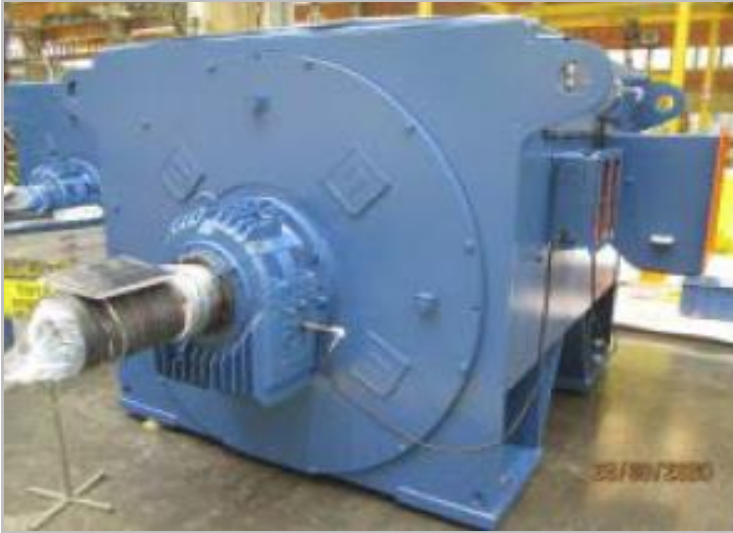
Figure 6 | SAG Mill Motor
