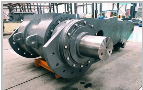
Figure 13 | Trial Assembly of Mill Feed Conveyor
