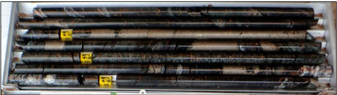
Figure 3: Photograph of sulphide intersection with massive, and semi-massive pyrrhotite from single hole MARD0094.
