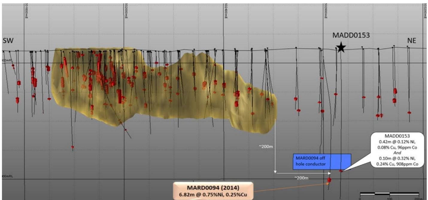
Figure 2: Long section of Maibele North resource (brown shape) plus extensional areas to the west and east.
