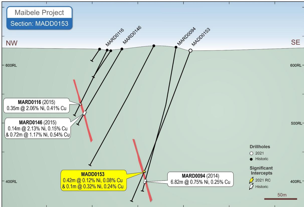
Figure 5: Cross section showing step out holes
