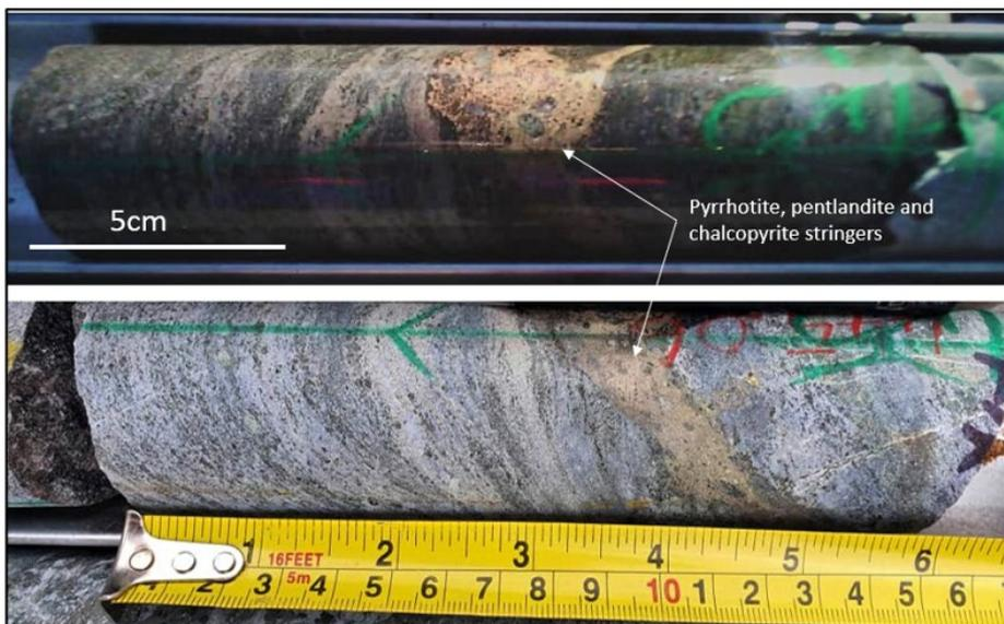
Figure 4: Examples of massive sulphide stringers from ~445m depth in MADD0153
