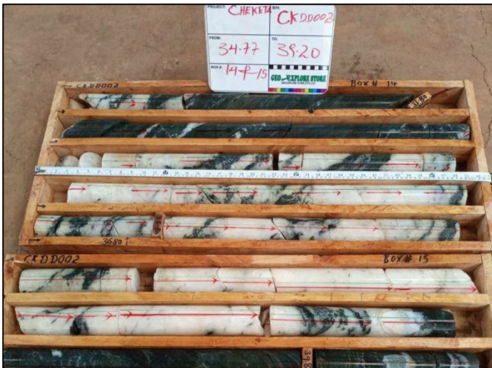
Figure 4 – Current drilling by Megado, drillhole CKDD002 (Contact Target) showing broad zones (ca. 5m interval) of quartz-tourmaline-pyrite veining
