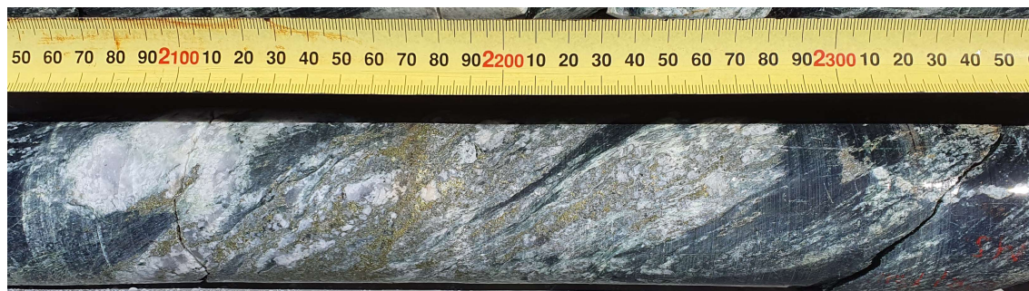
Figure 1 – 10-15cm quartz-carbonate-chalcopyrite (20%)-bornite (<1%) veining within FPDD004
