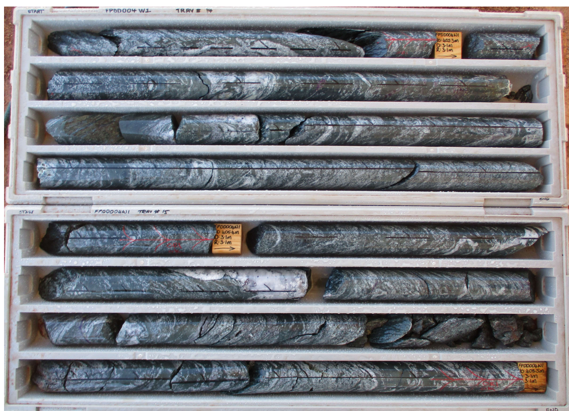
Figure 2 – Core tray photo (~401.5-408.5m) showing the mineralisation within FPDD004W1
