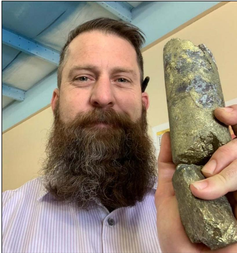
Figure 1 – Principal Geologist Brian Paull holding core from WT-21-06 (from 371.6m) which assayed 34.4% Cu, 367g/t Ag and 26.2g/t Au
