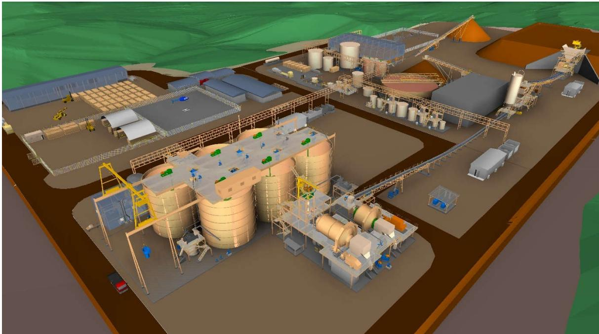
**Figure 2. Redesigned Stage 1 circuit incorporating provision for possible future expansion.**
