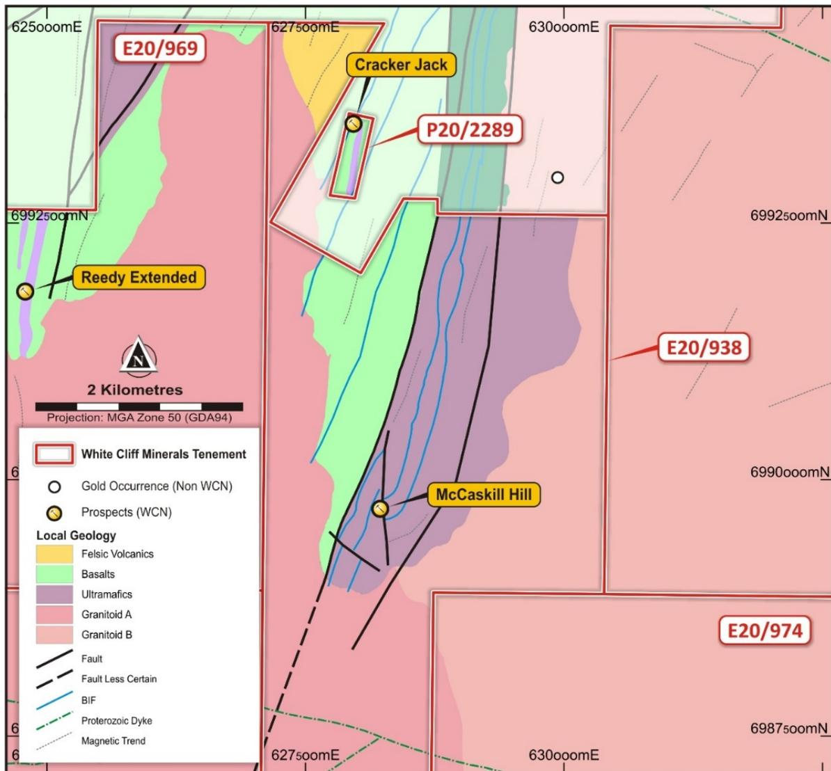
**Figure 4:** Cracker Jack and McCaskill Hill prospects over mapped geology, highlighting the extensive structural systems within the Company's tenement holding
