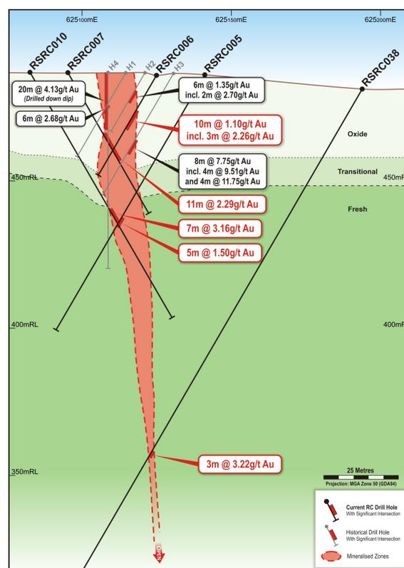
**Figure 5:** Depth extensions to mineralisation at the King Cole prospect
