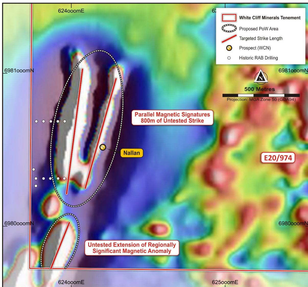
**Figure 7:** Nallan prospect over magnetics, highlighting the targeted strike length to be tested by first pass soil sampling
