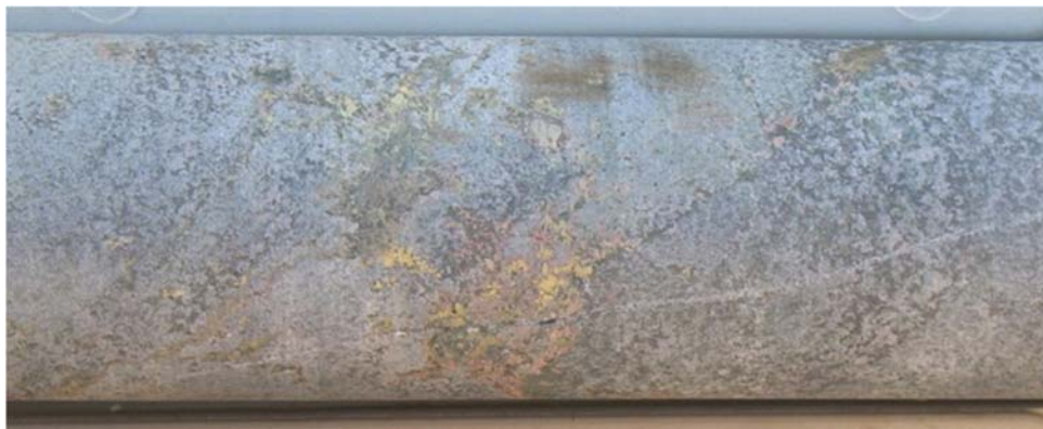
Photograph; FC2 Prospect: Drill core from MMA008 @ 193m DH. Pyrite and Chalcopyrite (ca.1%) in magnetite altered banded calc-silicate rock unit.
