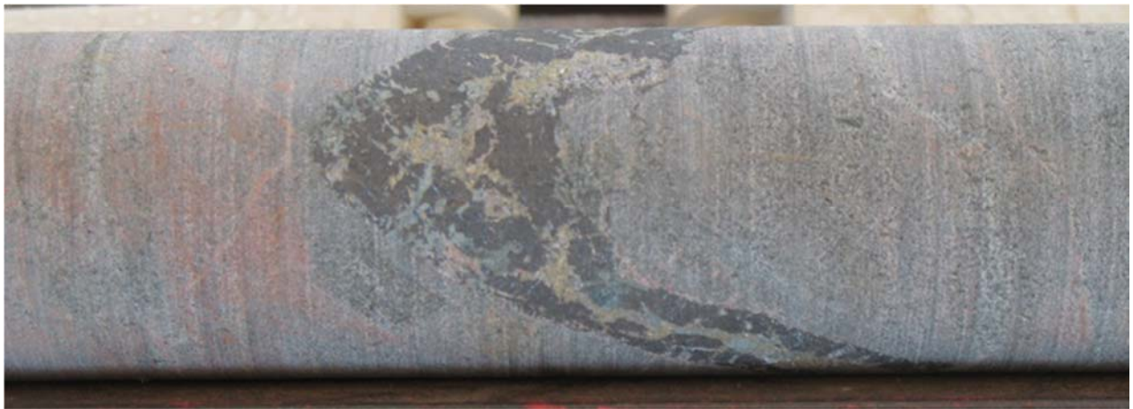
Photograph; FC2 Prospect: MMA007 drill core @ 130m. Magnetite-Actinolite-Pyrite-Chalcopyrite veining of Feldspar-altered mafic intrusive.
