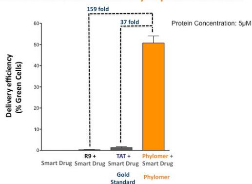
Split-GFP assay for measuring cytoplasmic Delivery using Different CPPs
