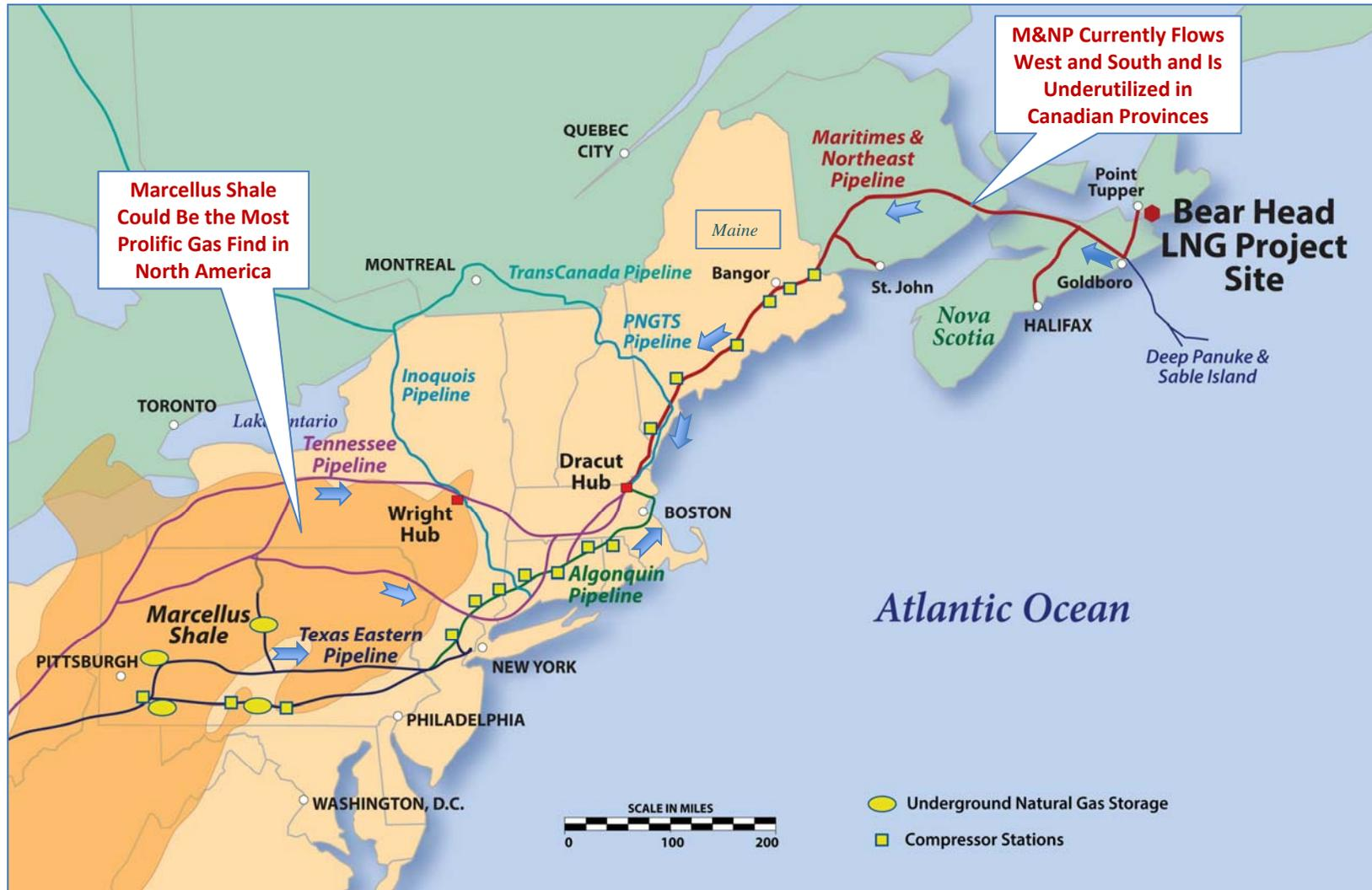
**Gas Supply to the Bear Head LNG Project requires construction of a gas transmission pipeline off the M&NP pipeline to deliver gas from Goldboro to the Bear Head LNG terminal site**
