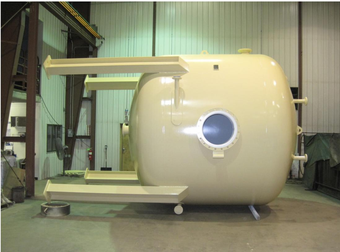
**Figure 3: Completed Ion Exchange Column for the CPP**
