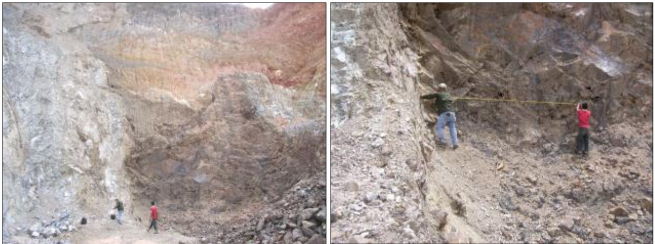
Figure 12: (L) Current Western Mining Face 13m Wide by 11m High and (R) Checking face width.
