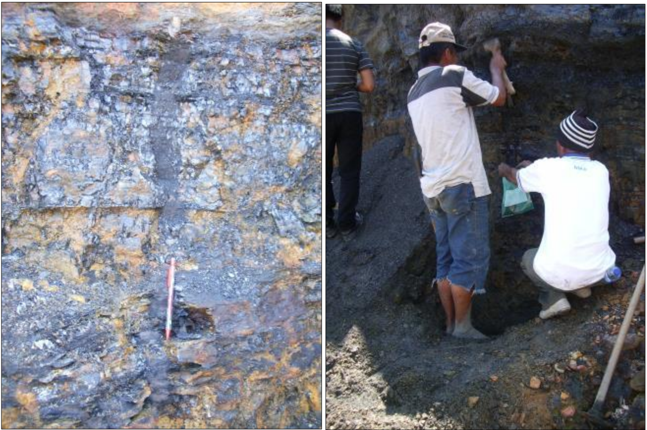
Figure 7: (L) WP904 – Sample TR02A Channel Sample of 40cm Anthracite Seam, (R) Sampling Black Shale Footwall Sample TR02B.
