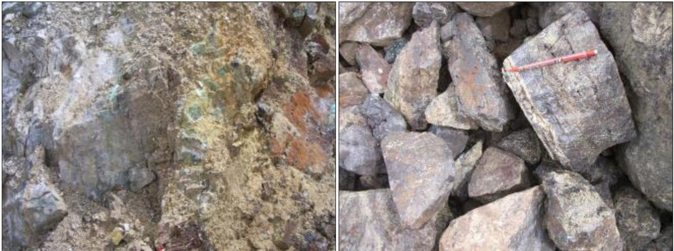
Figure 14: (L) Visible Malachite Staining in the Sheared Selvage – Sample Pit 2-2 and (R) Broken Massive Magnetite Material in floor of Mining Slot.
