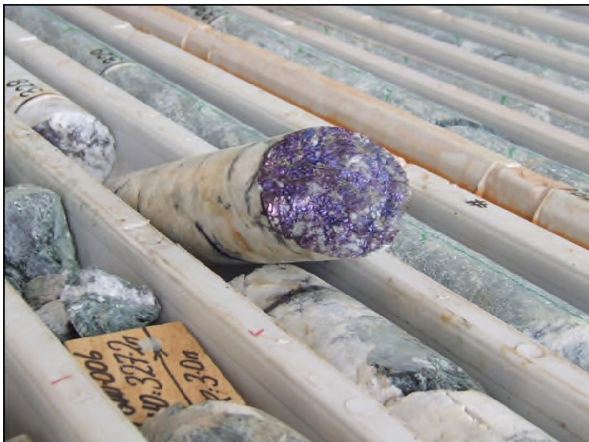
Figure 2: Bornite mineralisation in quartz lode breccias, drillhole FGDD006
