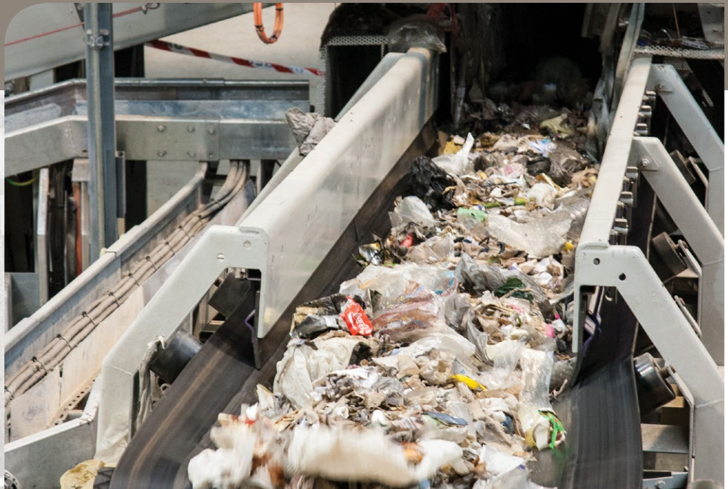
Coarse fraction on a belt conveyor prior to processing for recovery of plastics.
