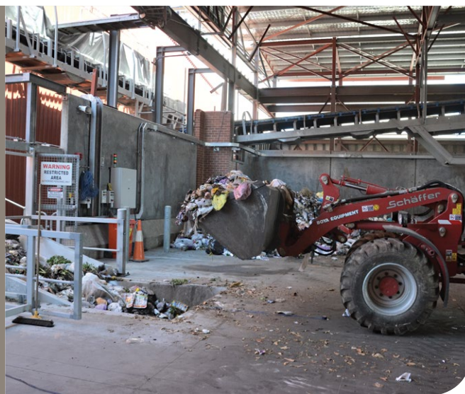
MSW on the tipping floor being introduced to the feed conveyor using a front end loader.
