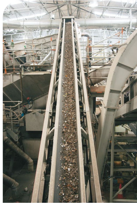
MRF belt conveyor with a fine organic fraction (<40mm) separated and recovered after processing through the trommel.
