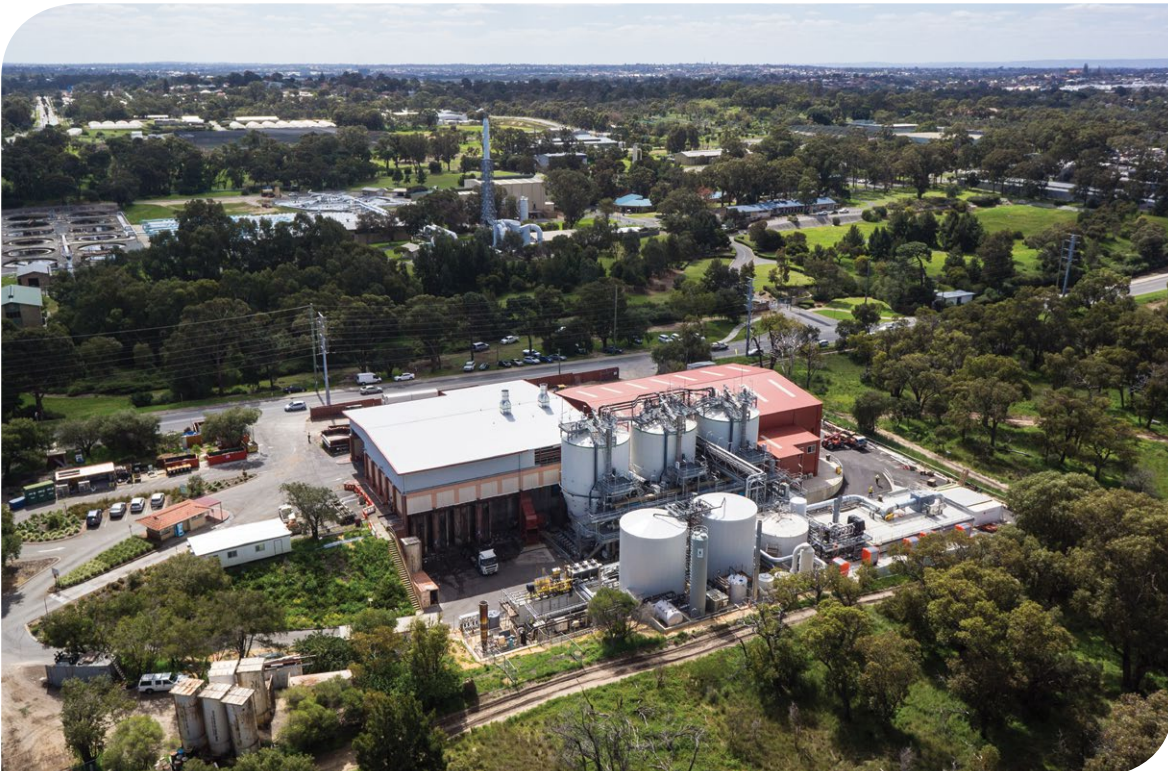
Aerial view of the JFR McGeough Resource Recovery Facility incorporating a 60,000 tpa AnaeCo™ AWT Plant, facing north east from Brockway Road. The facility is located around 6km from the Perth CBD.
