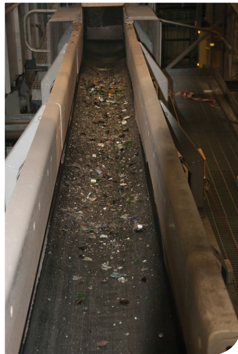
Separated glass and grit stream following processing of organic material through the WDS to remove contaminants.
