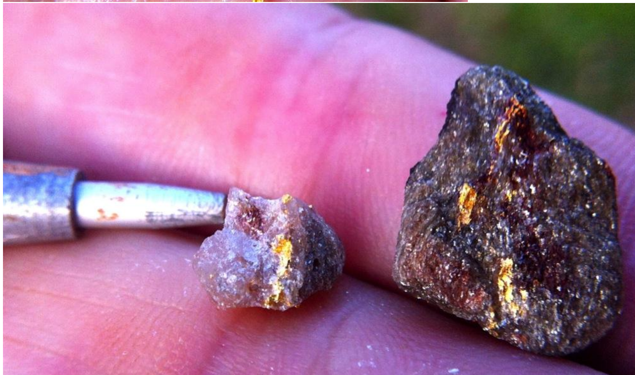
Figure 3a and 3b – Shows coarse visible gold up to 5mm strongly elongated parallel to the stretching lineation.
