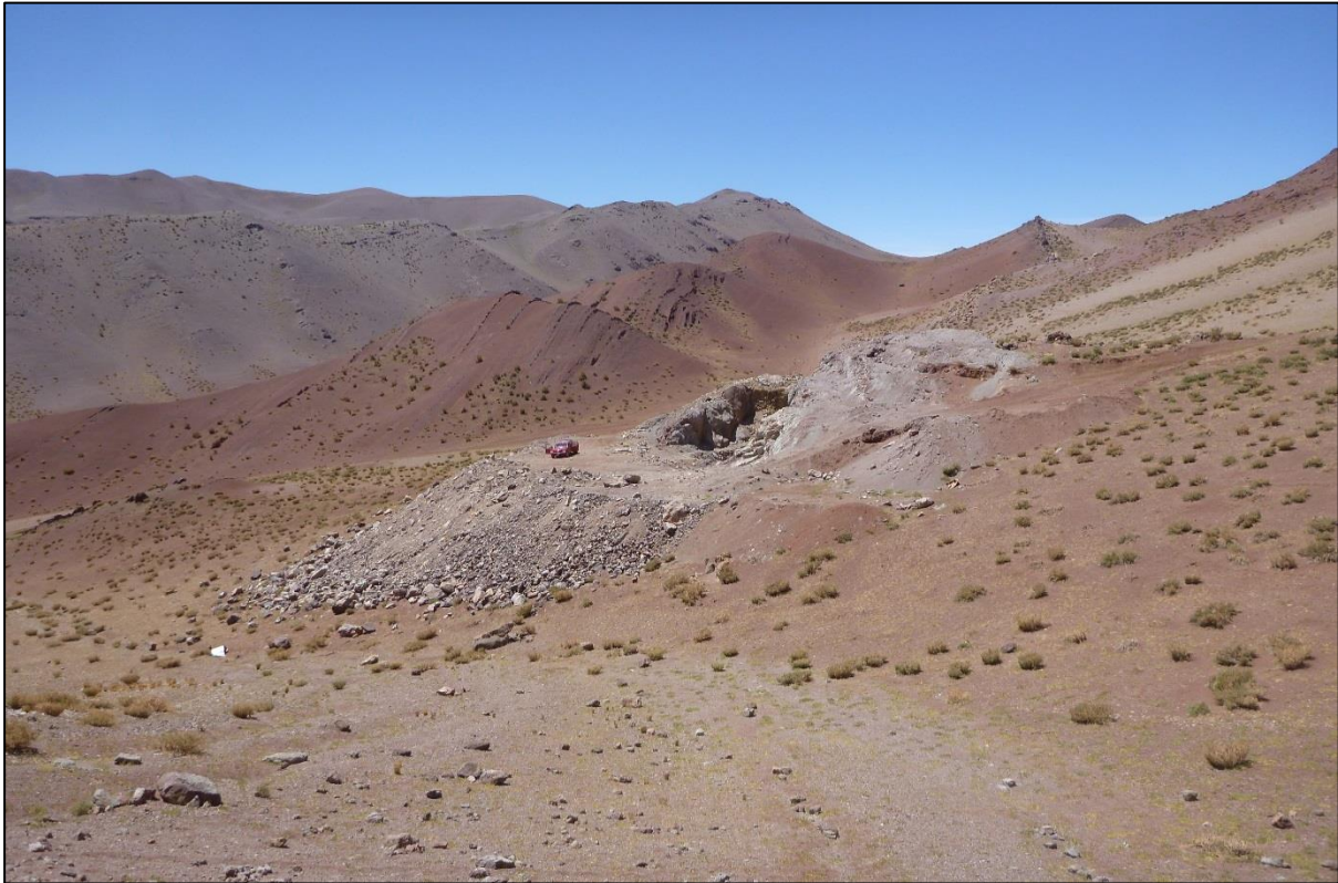
Figure 4: Excavation for secondary copper mineralisation, eastern mineralised unit
