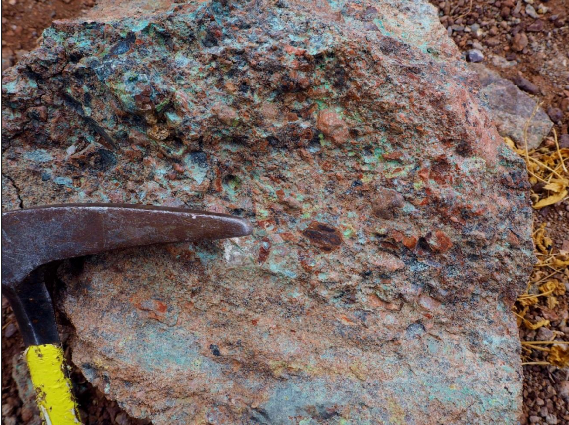
Figure 5: Pebble conglomerate with secondary copper, eastern mineralised unit
