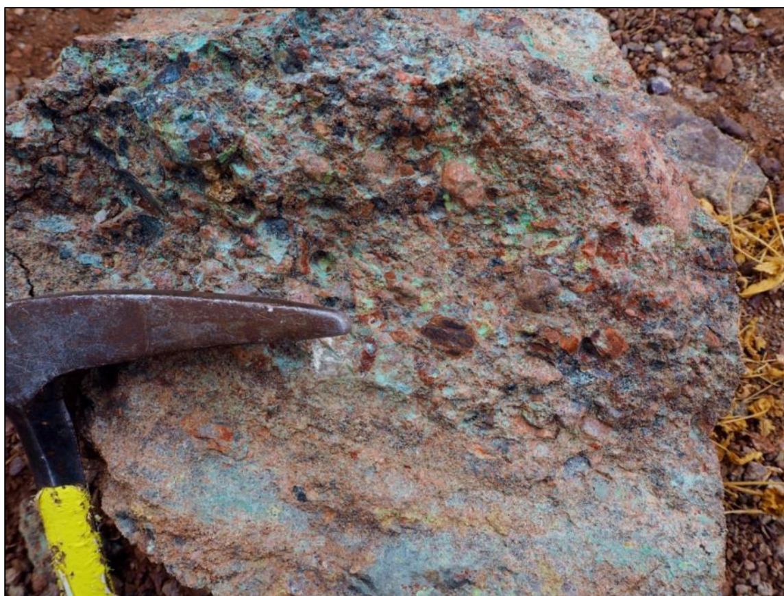
Figure 5: Pebble conglomerate with secondary copper, eastern mineralised unit
