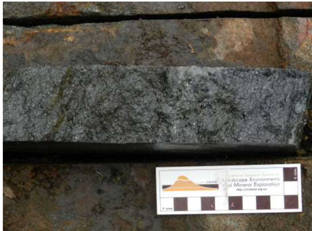
Figure 1: Flake graphite visible on underside of channel sample
