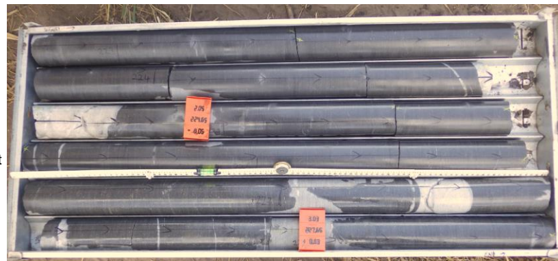
Graphite liberation as seen at surface on diamond drill hole GBND0005
