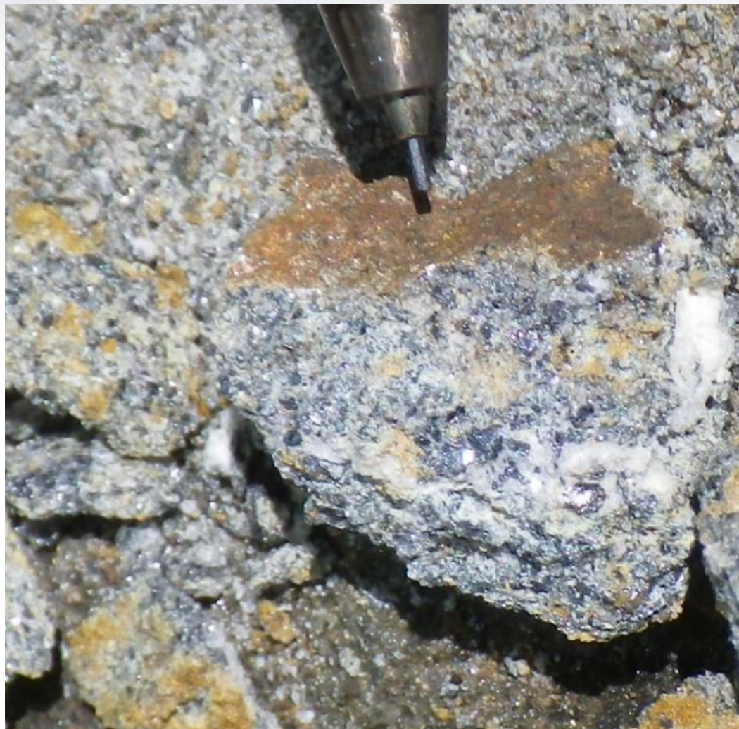
Close up image of the graphite-bearing quartzose schist found on exploration license 5304
