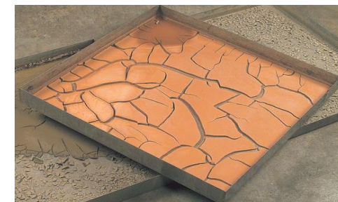
Screened slurry goethite 40% Leach feed grade 1.15% Ni
