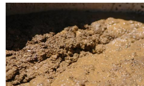
Screened rejects Silica fragments 60% Reject grade 0.4% Ni
