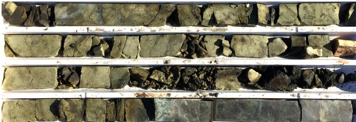
Figure 5: Massive chalcopyrite (primary copper sulphide) in hole TRBDD09: approximately 34m to 37.5m
