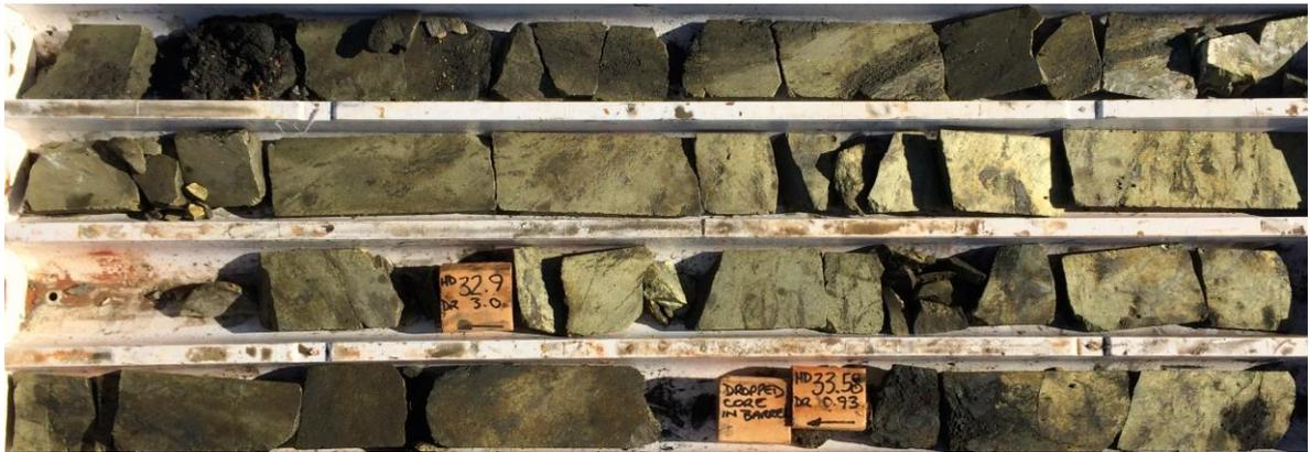
Figure 4: Massive chalcopyrite (primary copper sulphide) in hole TRBDD09: approximately 31m to 34m
