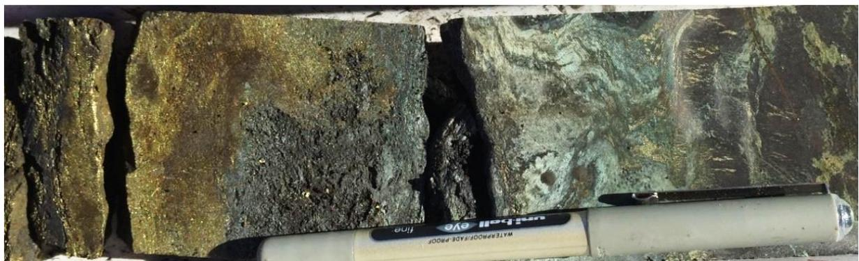
Figure 6: Massive chalcopyrite (primary copper sulphide): contact at 37m down hole TRBDD09
