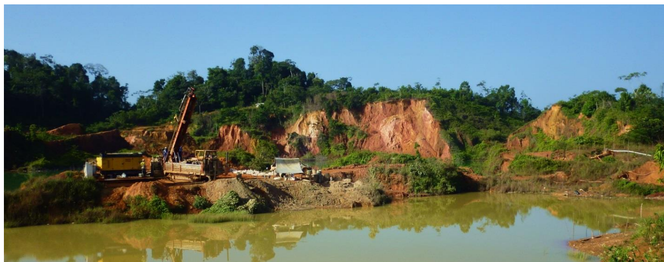
Figure 6 | 14 Mile Target: RC drilling at Gold Hill.
