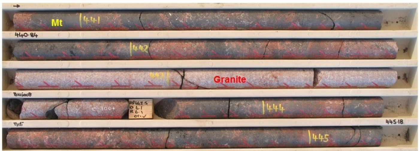
Photograph: Bronzewing Bore Prospect. Drill-core from BNG001 (441-445m) showing typical magnetite (black areas) + red-feldspar alteration of Wimberu Granite. Magnetite initially replaces quartz.
