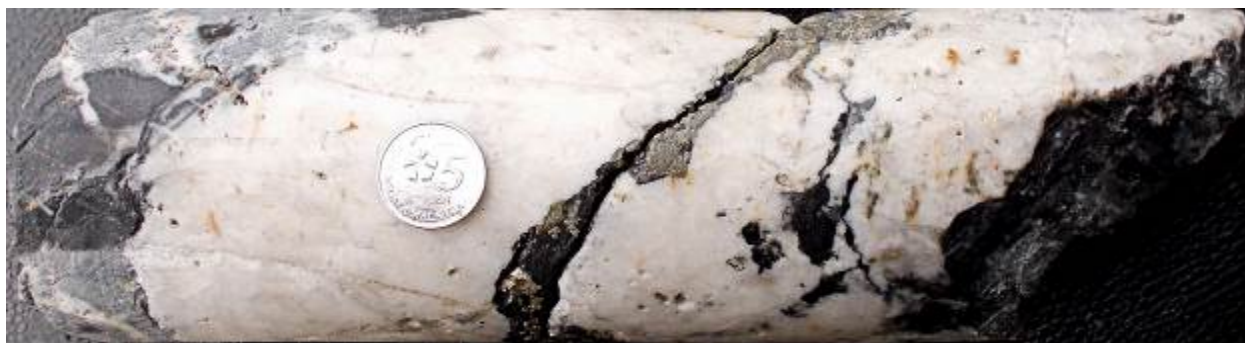
Close-up photograph from mineralised interval in LMD0010 (170.5m, 65.6ppm Au). Milky white massive sheared brecciated quartz vein with polymictic clasts (carbonaceous shale, shale, sandstone with minor epidote). The vein consists of quartz-carbonate-limonite-pyrite, up to 3% pyrite.
