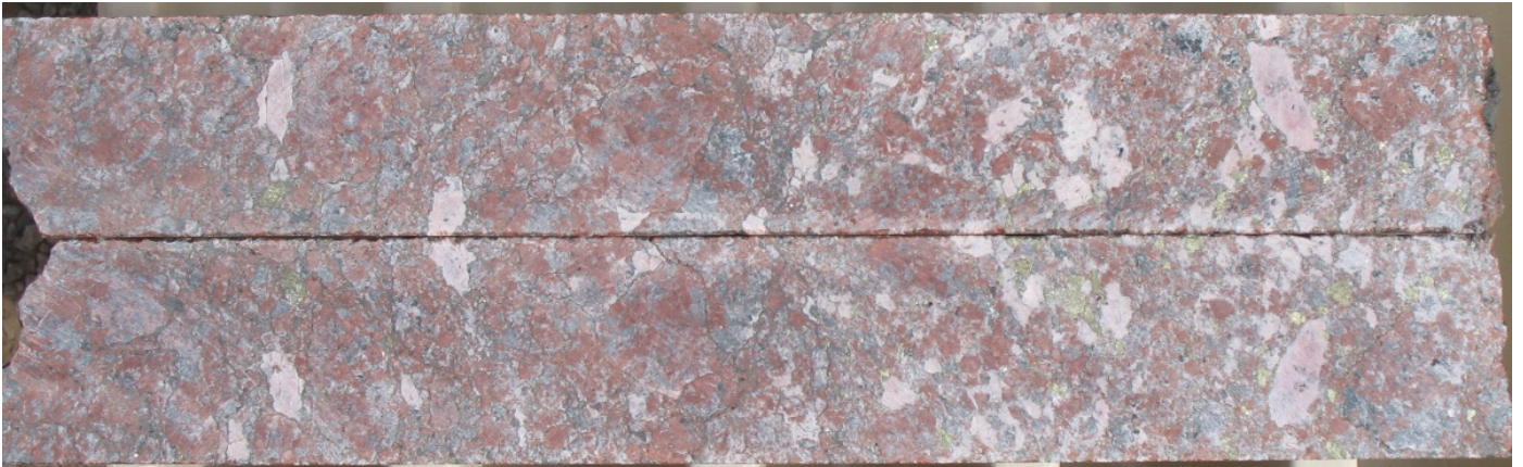
Photograph: Bronzewing Bore Prospect. Drill-core from BNG001 at 600-600.3m (sawn section) showing carbonate-infill breccia developed in Wimberu Granite. This section contains ca 4% chalcopyrite.
