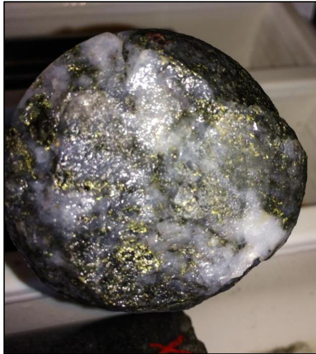
**Figure 2:** Pyrite and chalcopyrite in quartz vein aligned with foliation in a garnet bearing granulite gneiss (14SHDD06 456.2m)
