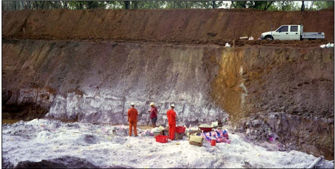
Figure 4 Test mining of magnesite at Winchester deposit. Crew standing on top of the magnesite mineralisation. Deposit has only few meters of overburden and a low strip ratio.
