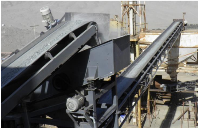
Picture 2: Dry Commissioning of the Crushing Circuit
