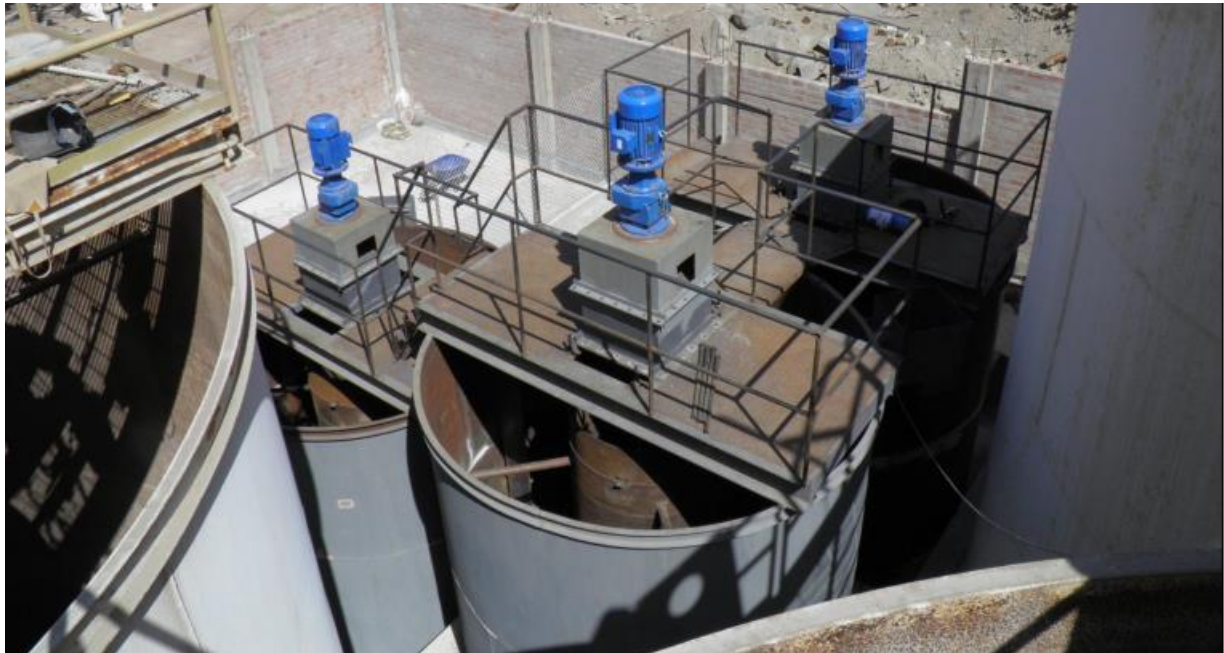
Picture 4: New carbon tanks installed prior to painting and wet commissioning.
