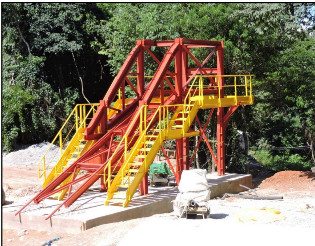
Figure 1. Erected headframe for haulage of material up the Main Incline Shaft at Cascavel.
