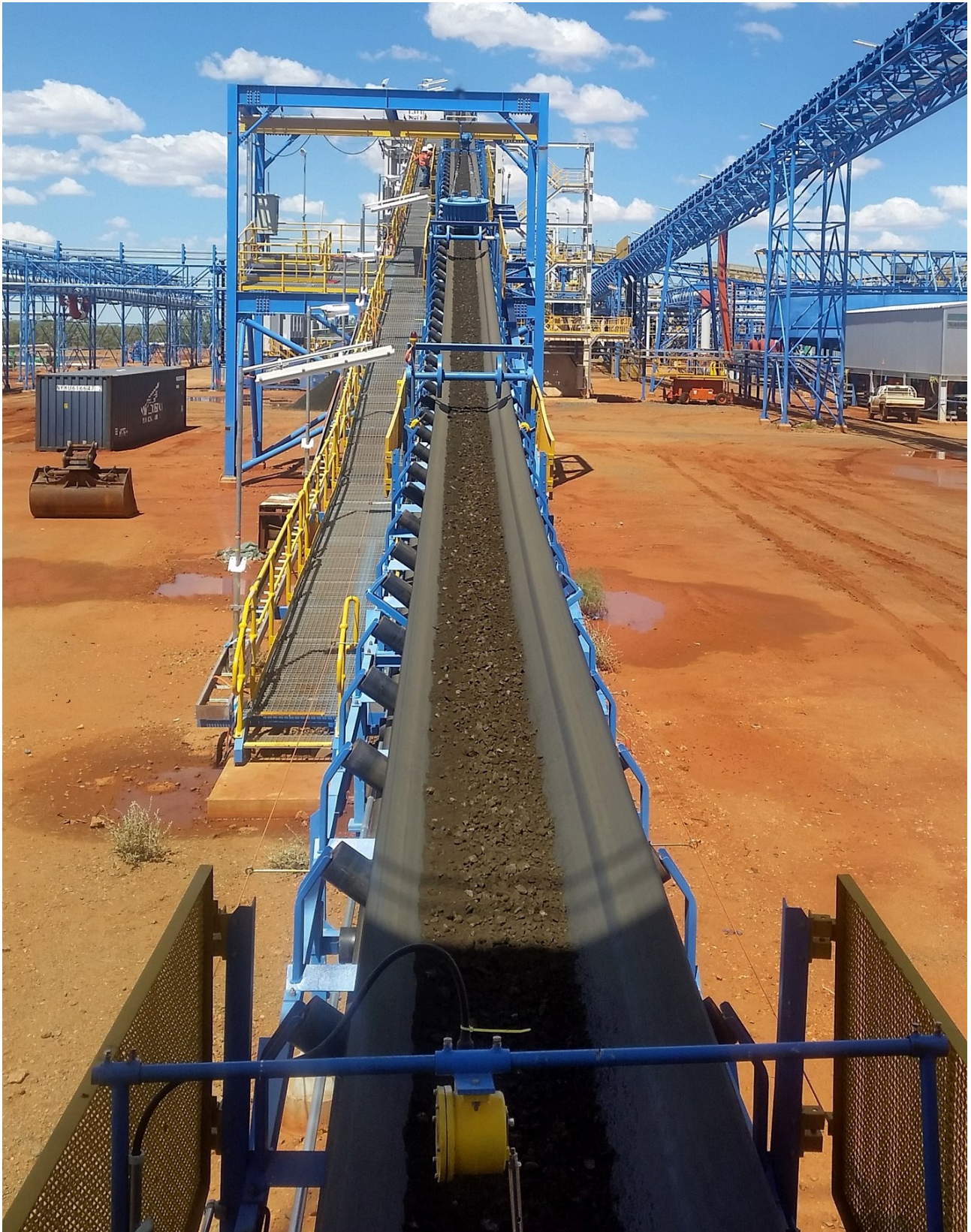
Figure 3: First feed to conveyor 3 (feeds to HPGR - structure behind the conveyor in background).
